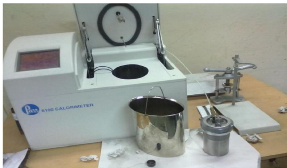
Plate 3.3: Isothermal bomb calorimeter
