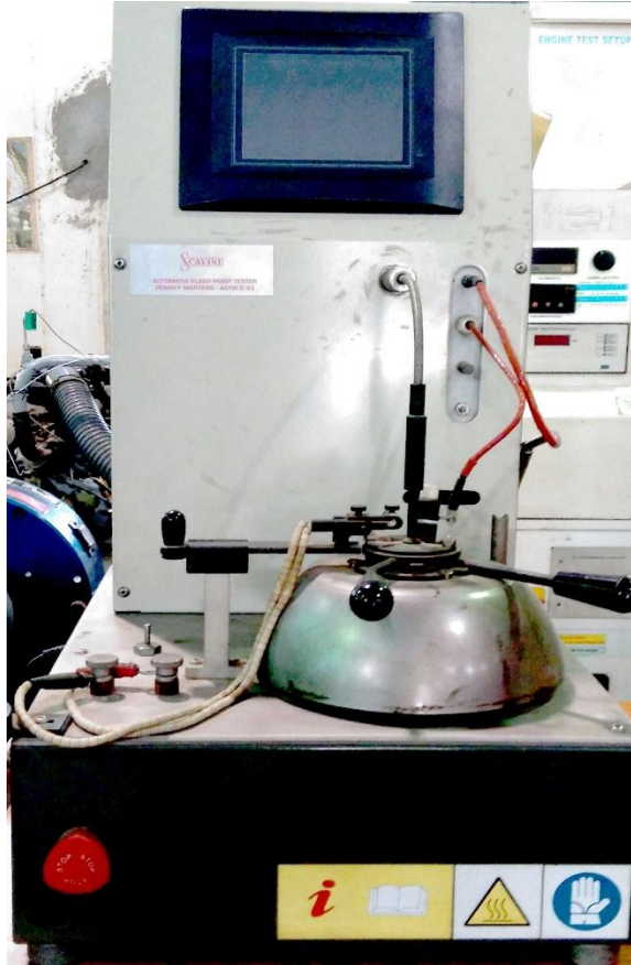
Plate 3.4: Pensky Marten's automatic flash point apparatus
