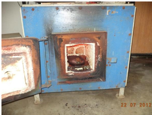
Mobile Phones PCB put to Roasting High Furnace
