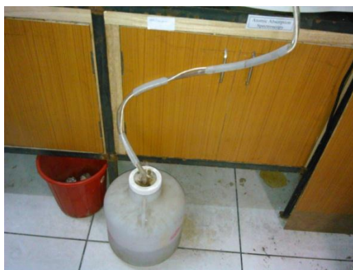
Waste Trough of FAAS
