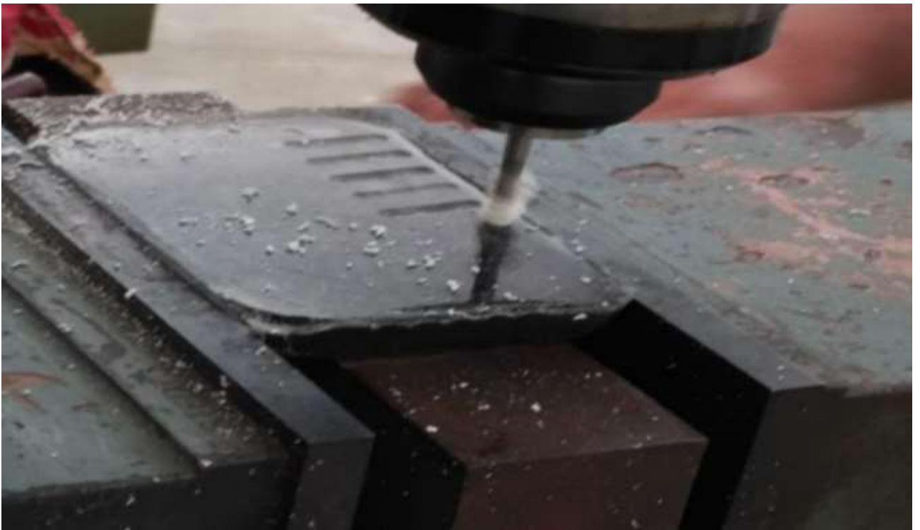
Fig 3.6. Machining on the GO-epoxy Sample
