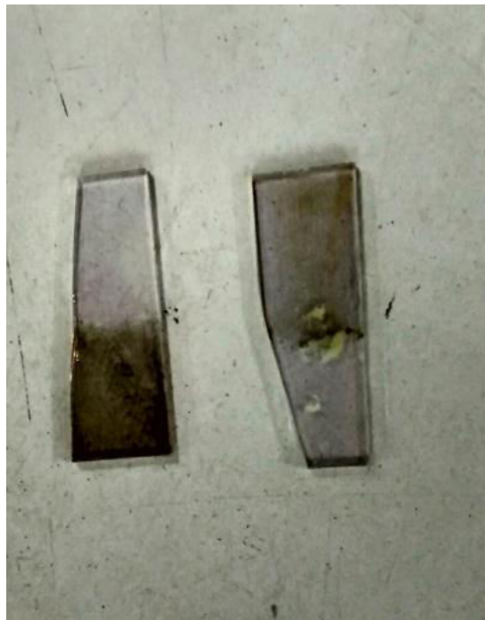
Fig 19: Deposited film of nanocomposite over ITO coated glass
