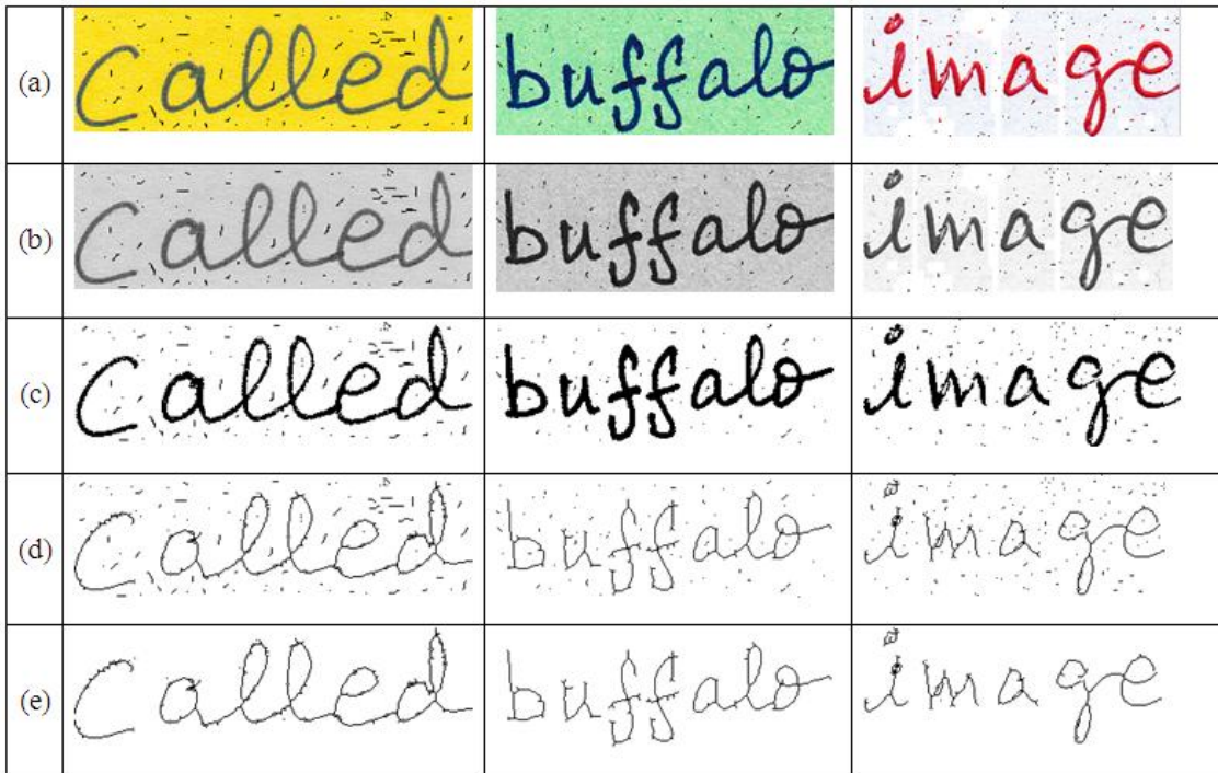
Fig.3.17 Word Image Preprocessing (a) Input Scanned Word Images; (b) Word Images after Gray Scale Intensity Threshold; (c) Word Images in Binary Format; (d) Word Images after Thinning; (e) Cropped Word Images after Noise Removal
