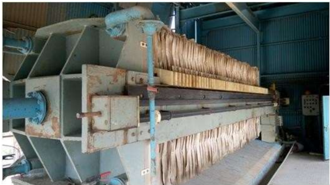
Figure 21: Filter press for separating suspended soil from water.
