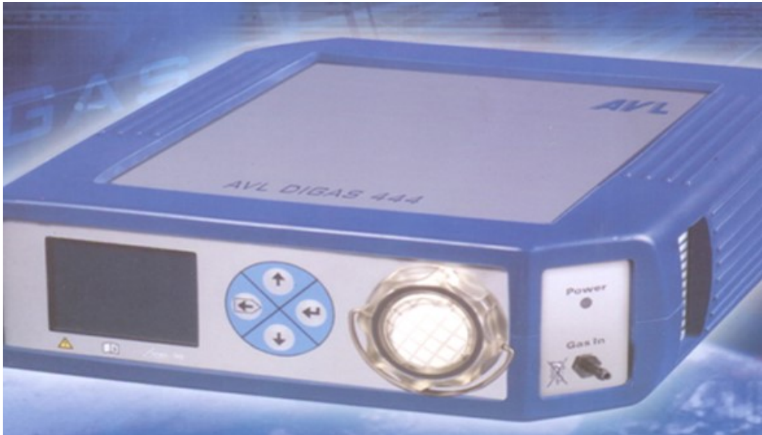
Fig. 3.3 Front view of the auto exhaust analyzer set up
