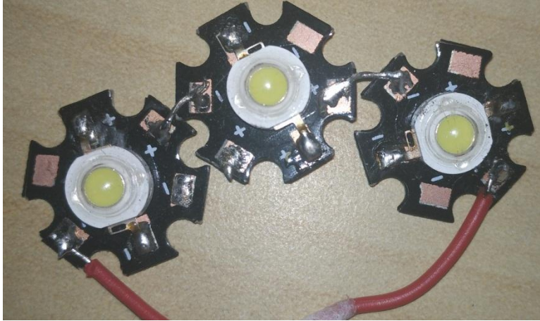
Fig.4.15 Selected power LEDs with heat sink
