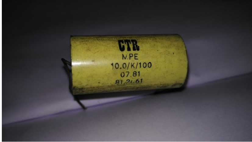
Fig.4.2 Chosen 10mfd 100V unpolarized film capacitor
