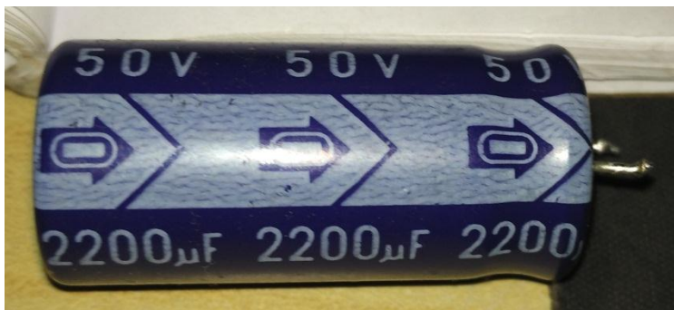
Fig.4.5 Chosen 2200mfd 50V polarized capacitor
