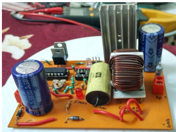
Fig.4.14 PCB after soldering all components
