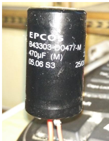
Fig.4.4 Chosen 470mfd 200V polarized capacitor
