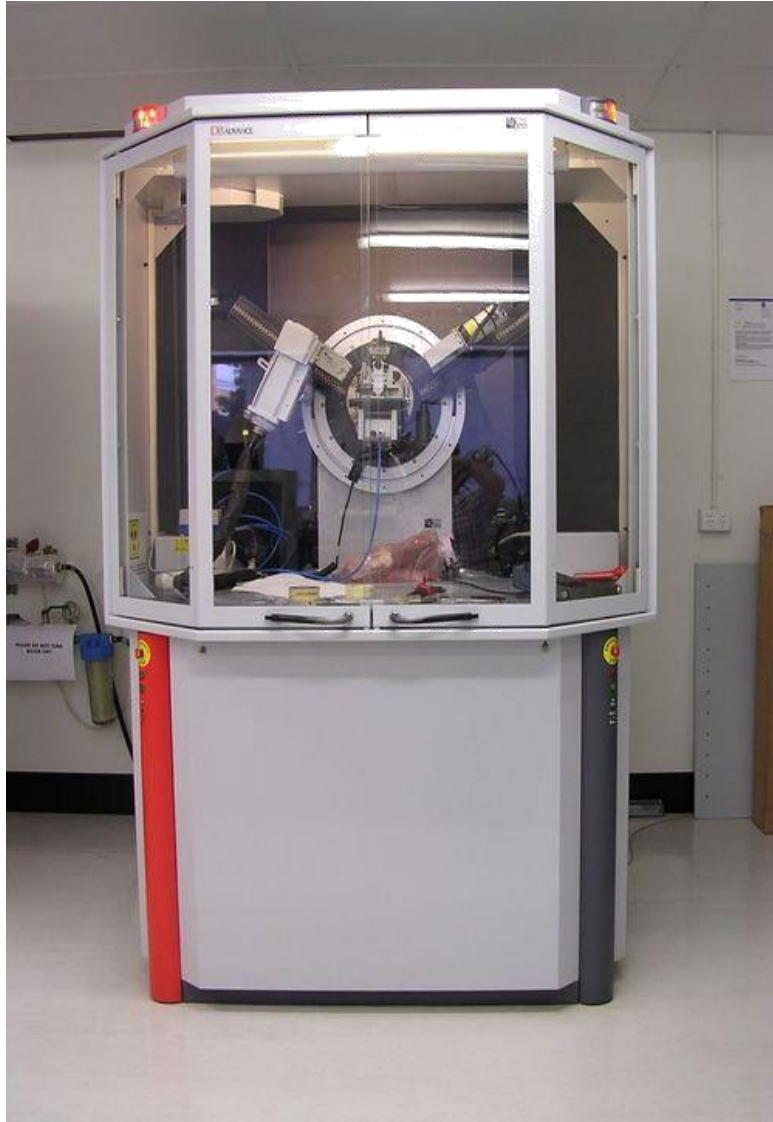
Figure 3.1 – Schematic of XRD machine[21]
