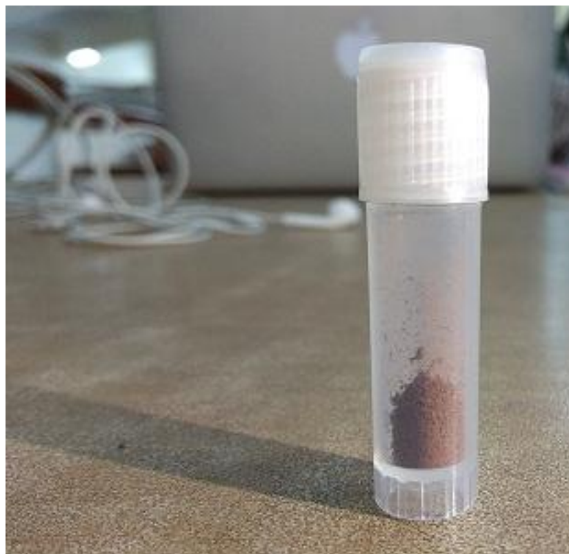
Fig.3.1 synthesized LMO nano material by electro-spinning
