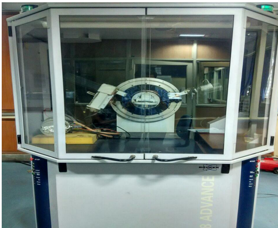
Fig 4.2 X-ray diffraction equipment used in the XRD characterization of LMO
