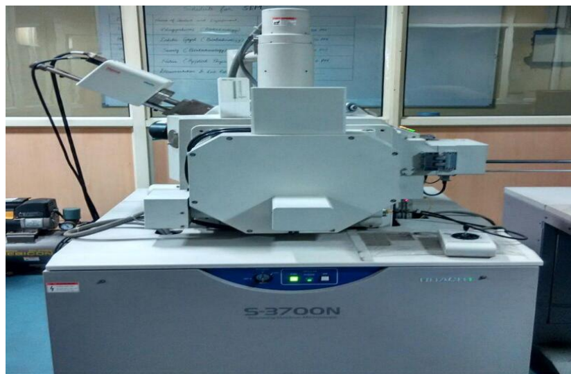
Fig 4.4 Scanning electron microscope equipment used in the SEM characterization of LMO
