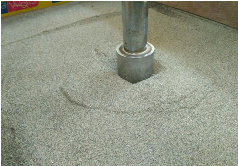
Figure 11 Shear failure of Yamuna sand at 5cmX5cm sq. plate
