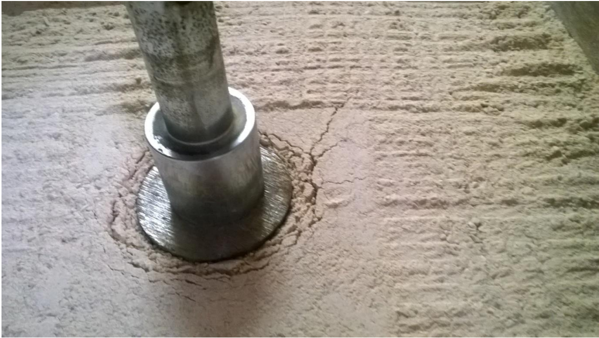
Figure 20 Shear failure of Badarpur sand under 7.5cm circular footing
