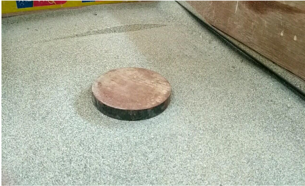
Figure 12 7.5 cm circular surface footing
