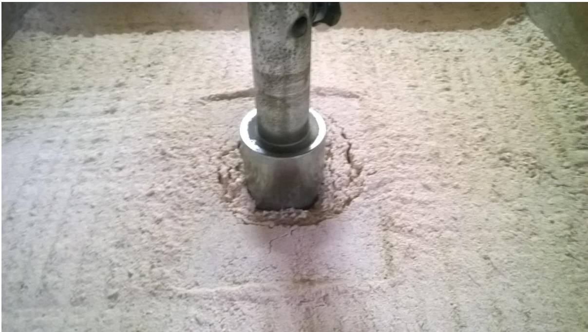
Figure 21 Shear failure of Badarpur sand under 5cm circular footing
