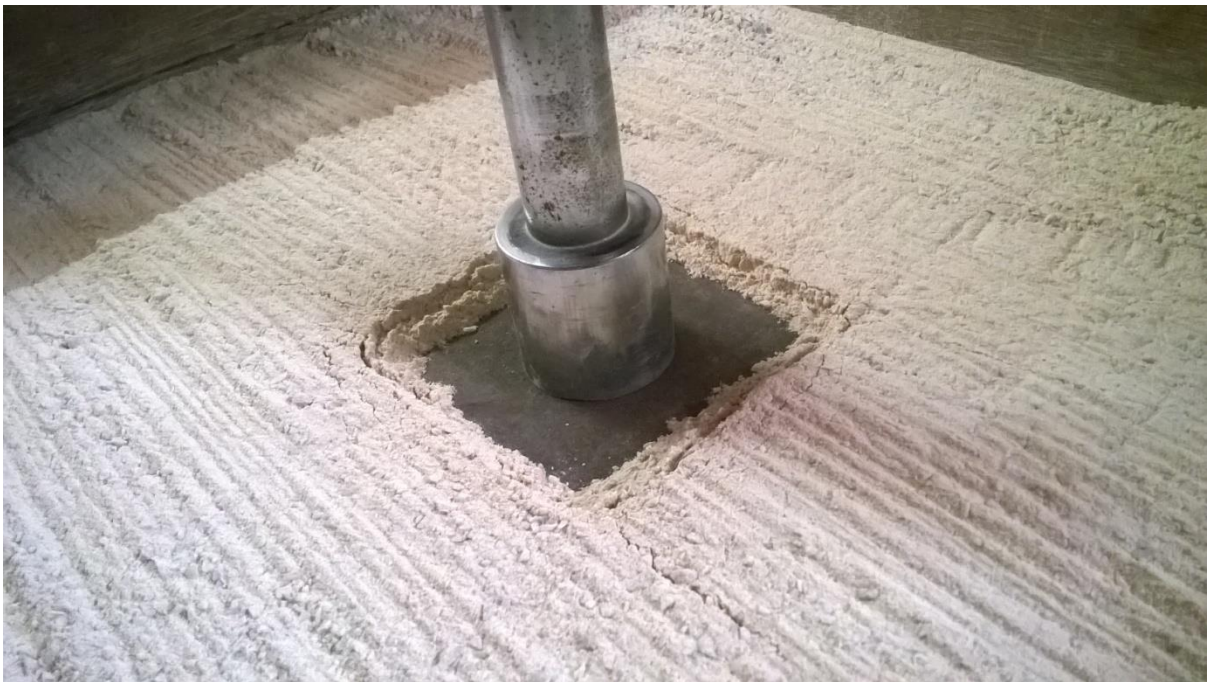
Figure 17 Shear failure of Badarpur sand under 10cmX10cm footing
