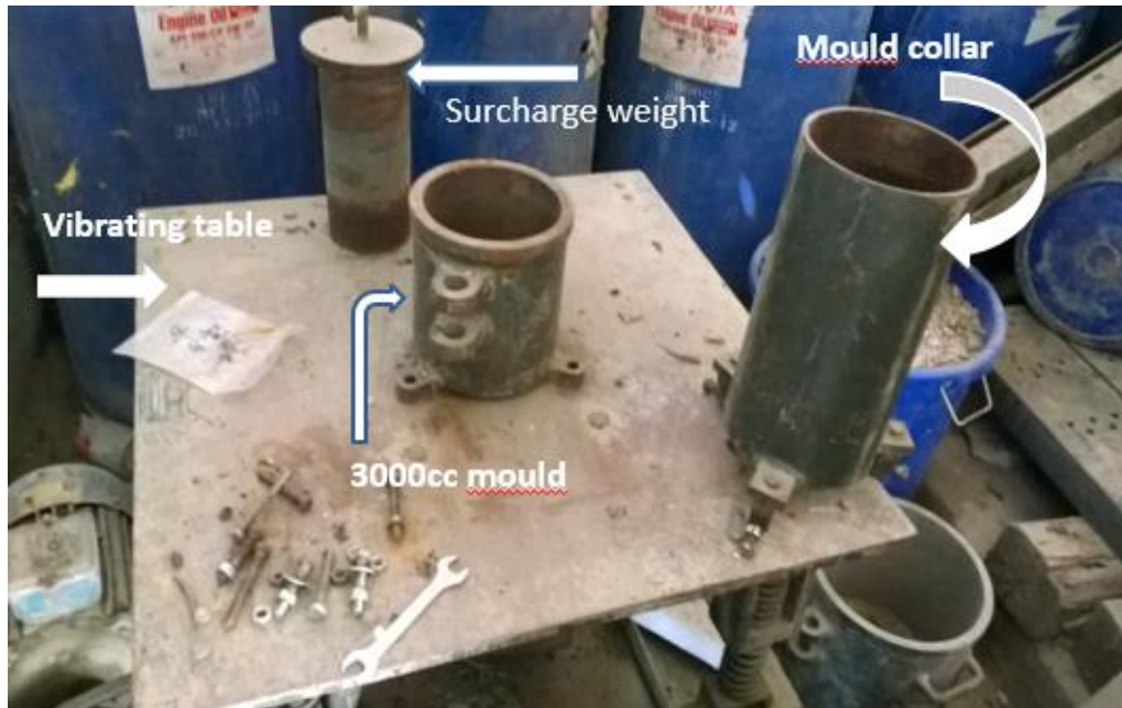
Figure 8 Relative density test apparatus
