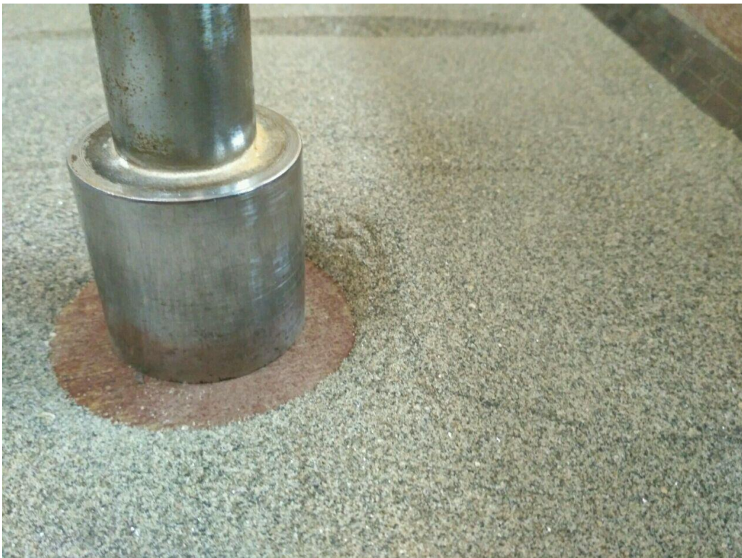
Figure 13 Shear failure on 7.5cm circular footing
