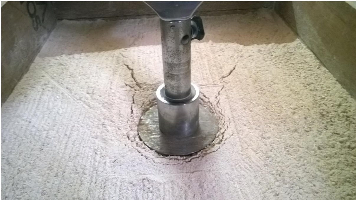
Figure 19 Shear failure of Badarpur sand under 10cm circular footing
