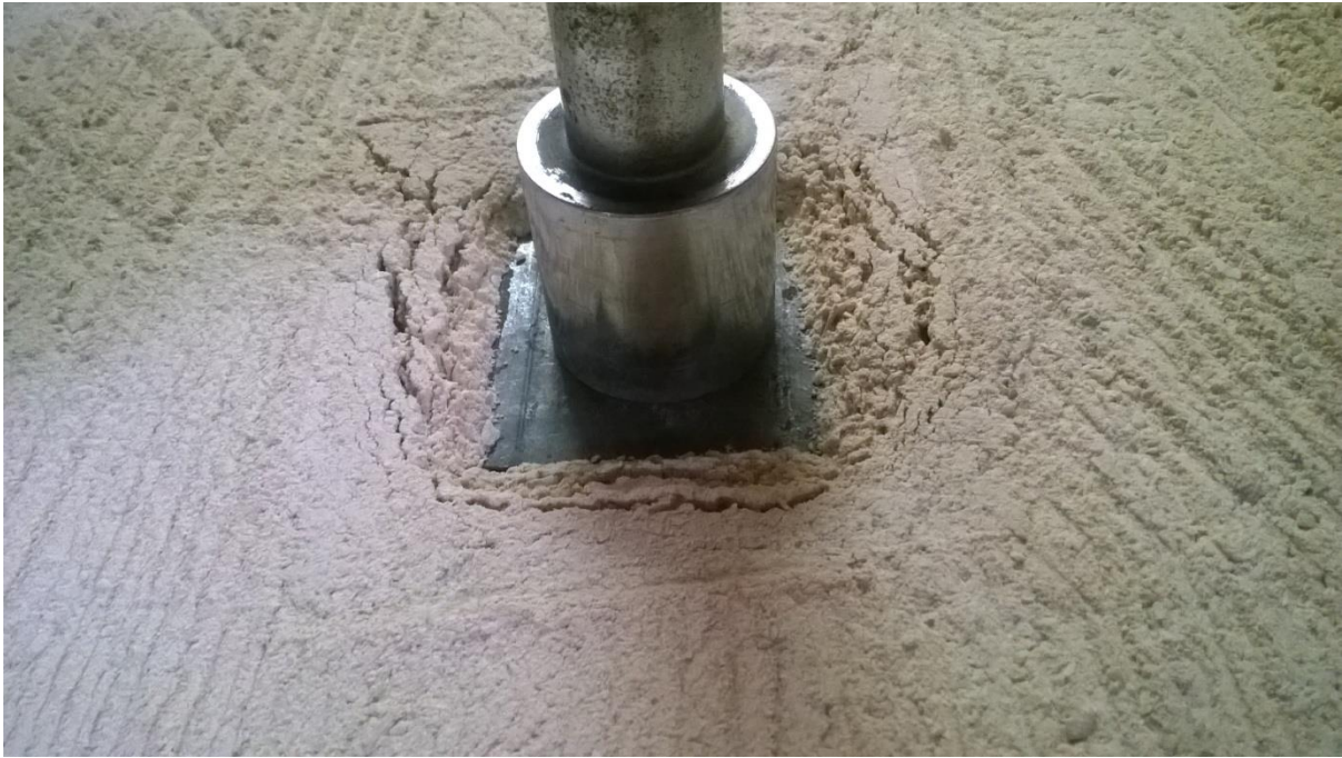
Figure 18 Shear failure of Badarpur sand under 8cmX8cm footing
