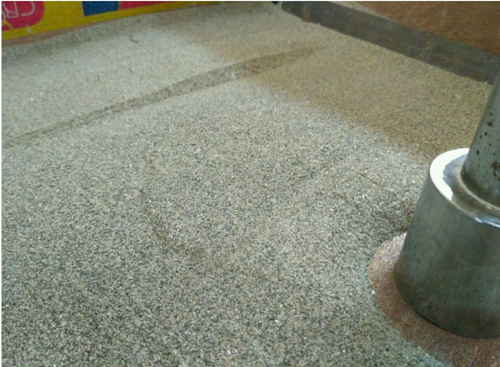
Figure 14 Shear failure of Yamuna sand under 7.5cm circular footing
