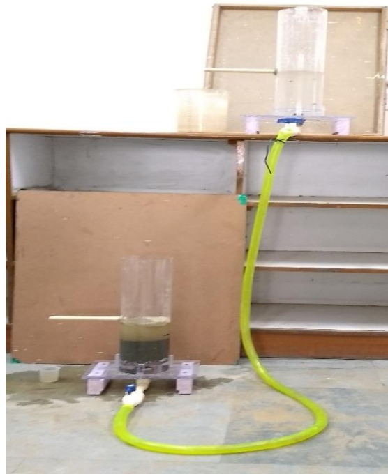
Fig 4.6 determination of permeability of Yamuna sand.
