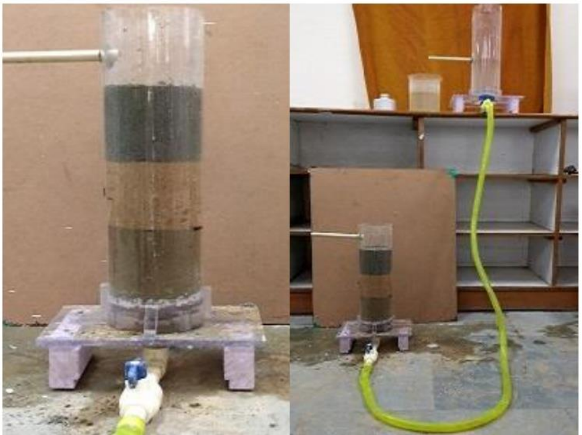
Fig 4.8. Experimental setup for determination of permeability of stratified soil
