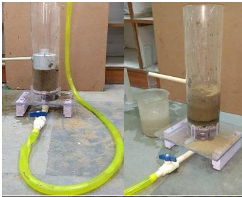
Fig. 4.7 Determination of permeability of DTU soil.
