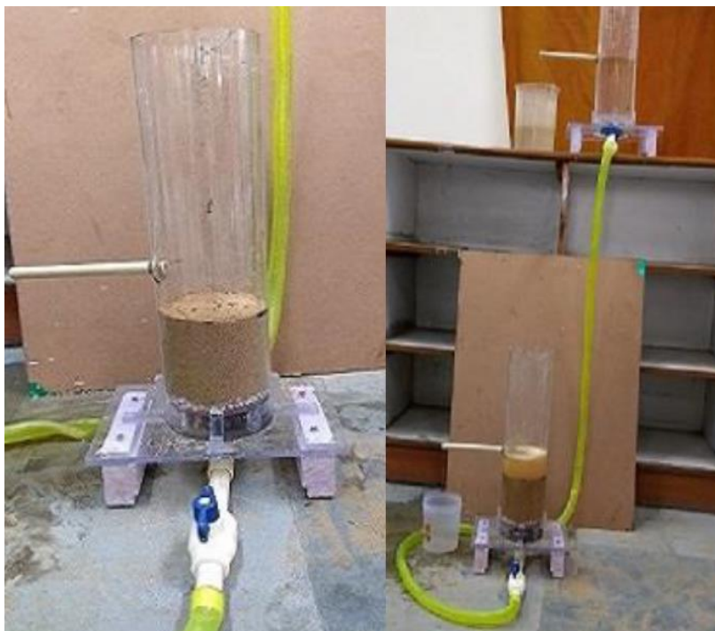
Fig.4.5 Experimental setup for determination of permeability of Badarpur sand
