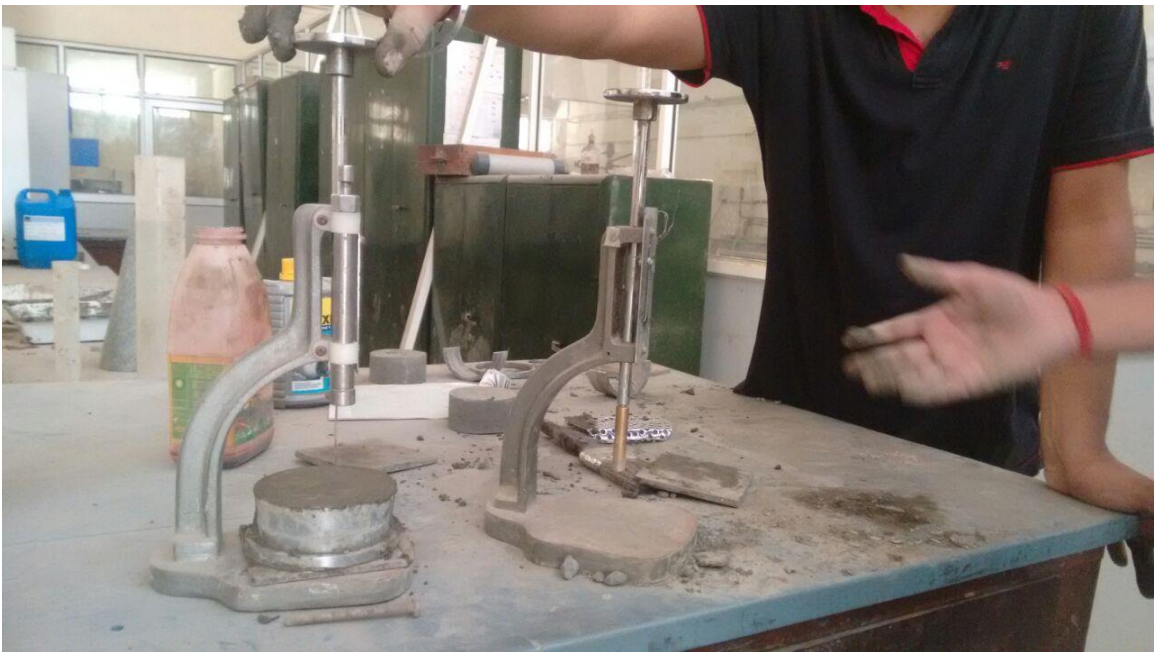
Fig 3: Test for Normal consistency
