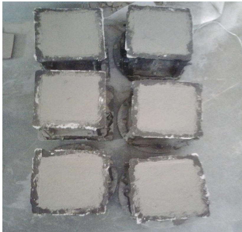
Fig 5: Concrete cubes casted in the mould
