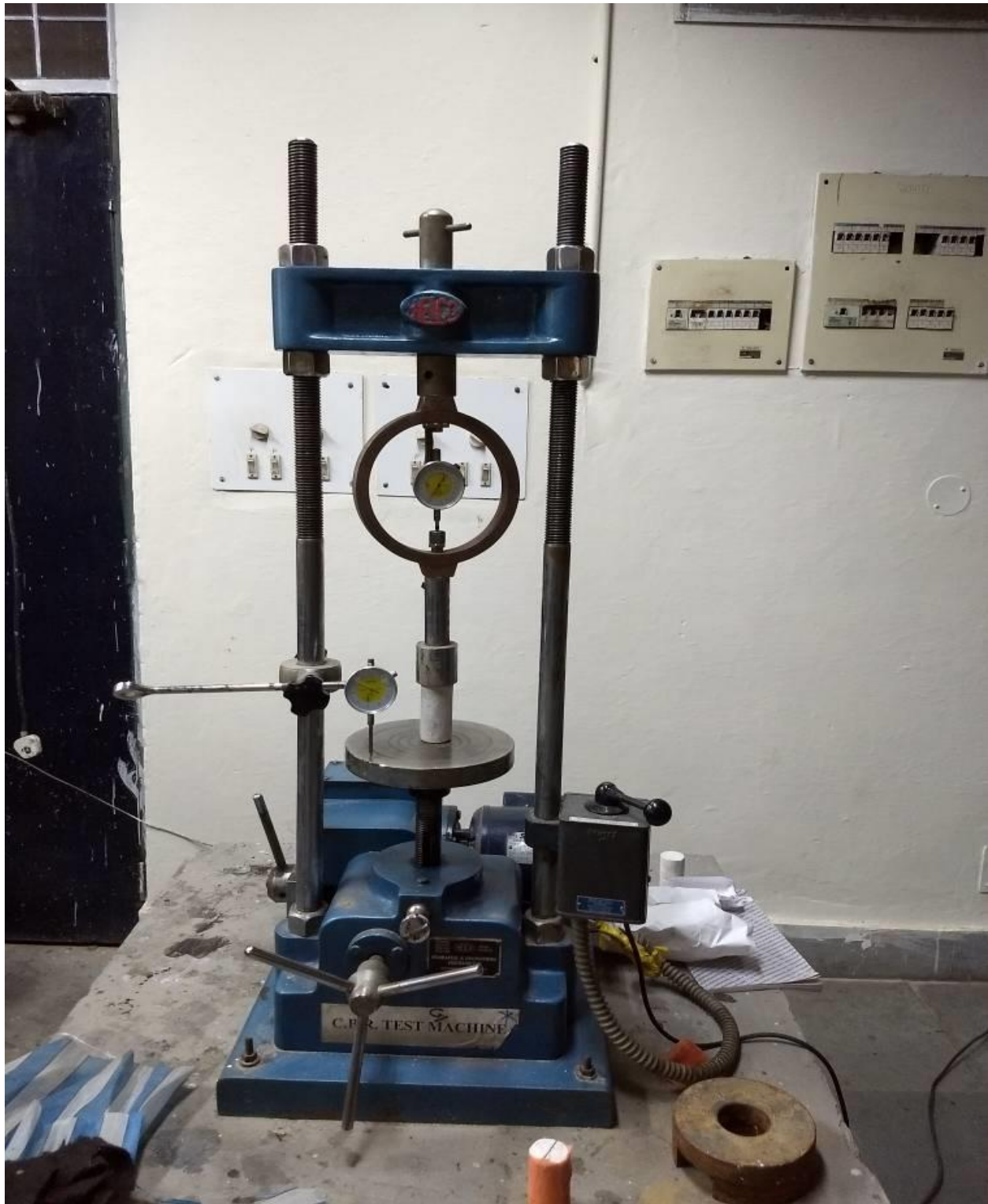
Figure 3.1.2: Uniaxial compression test for intact rock specimen
