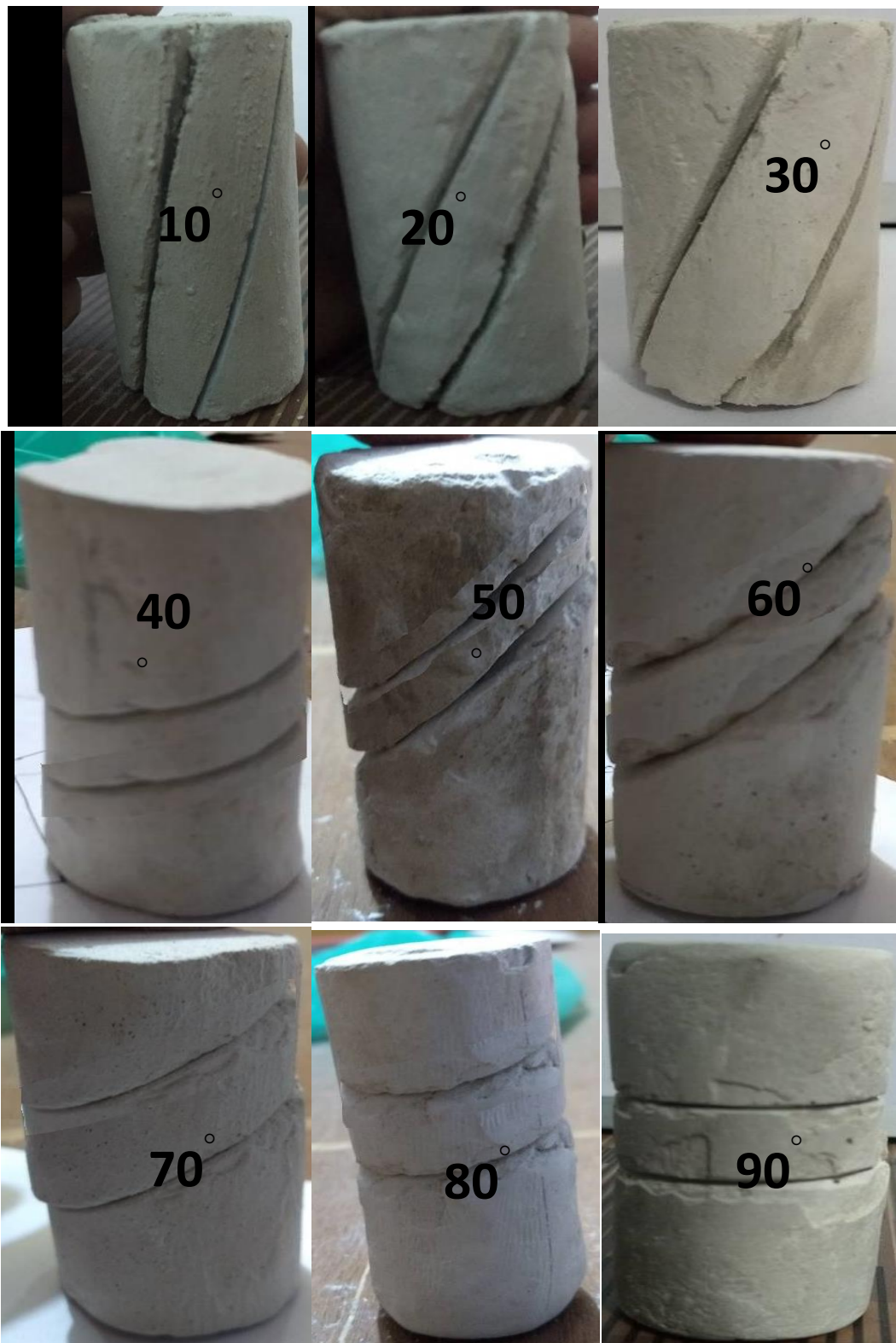
Figure 3.1.6: Types of joints studied in plaster of paris specimens and sand- plaster of paris mix specimens (double jointed specimens are shown here)
