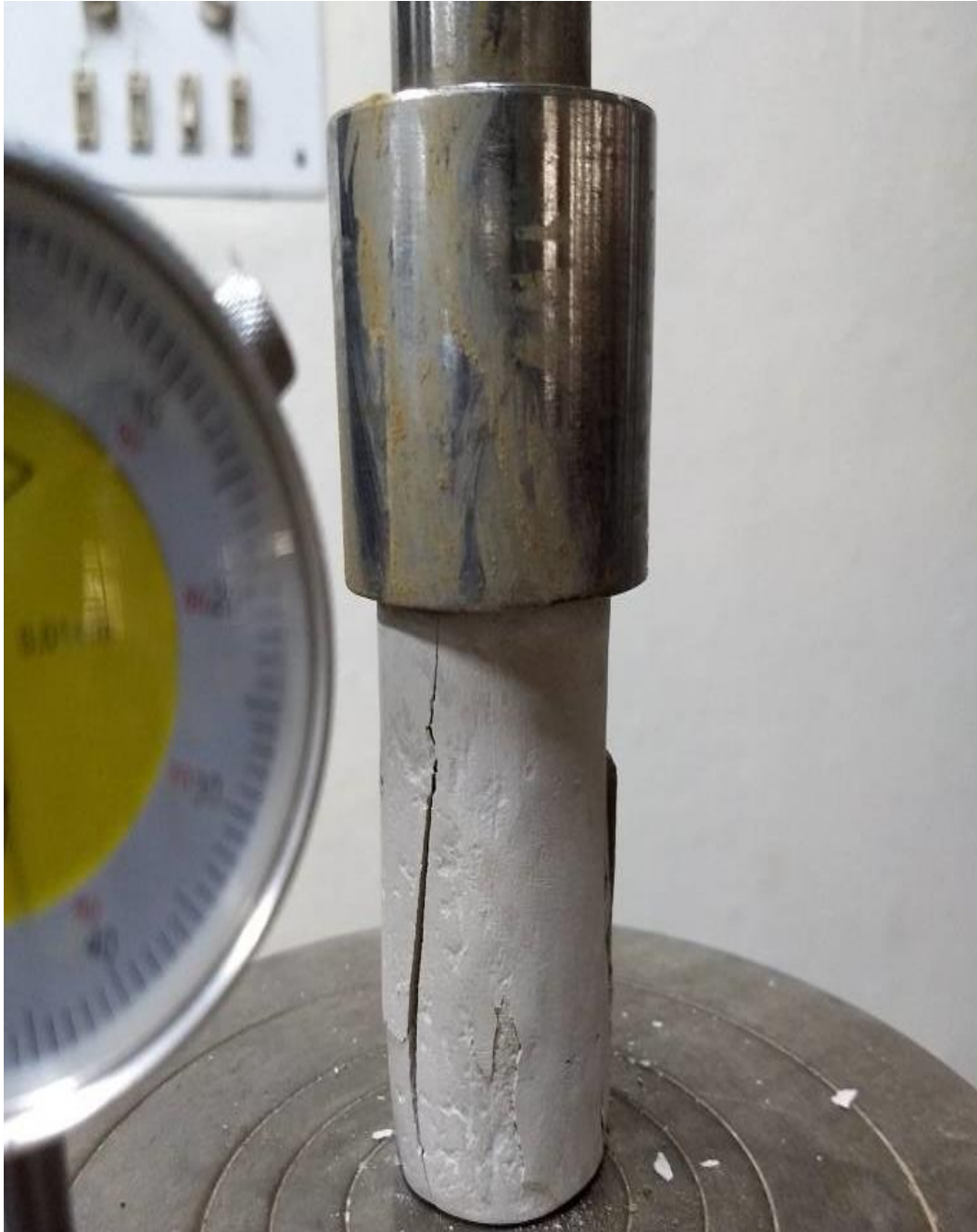
Figure 3.1.4: Failure of intact specimen
