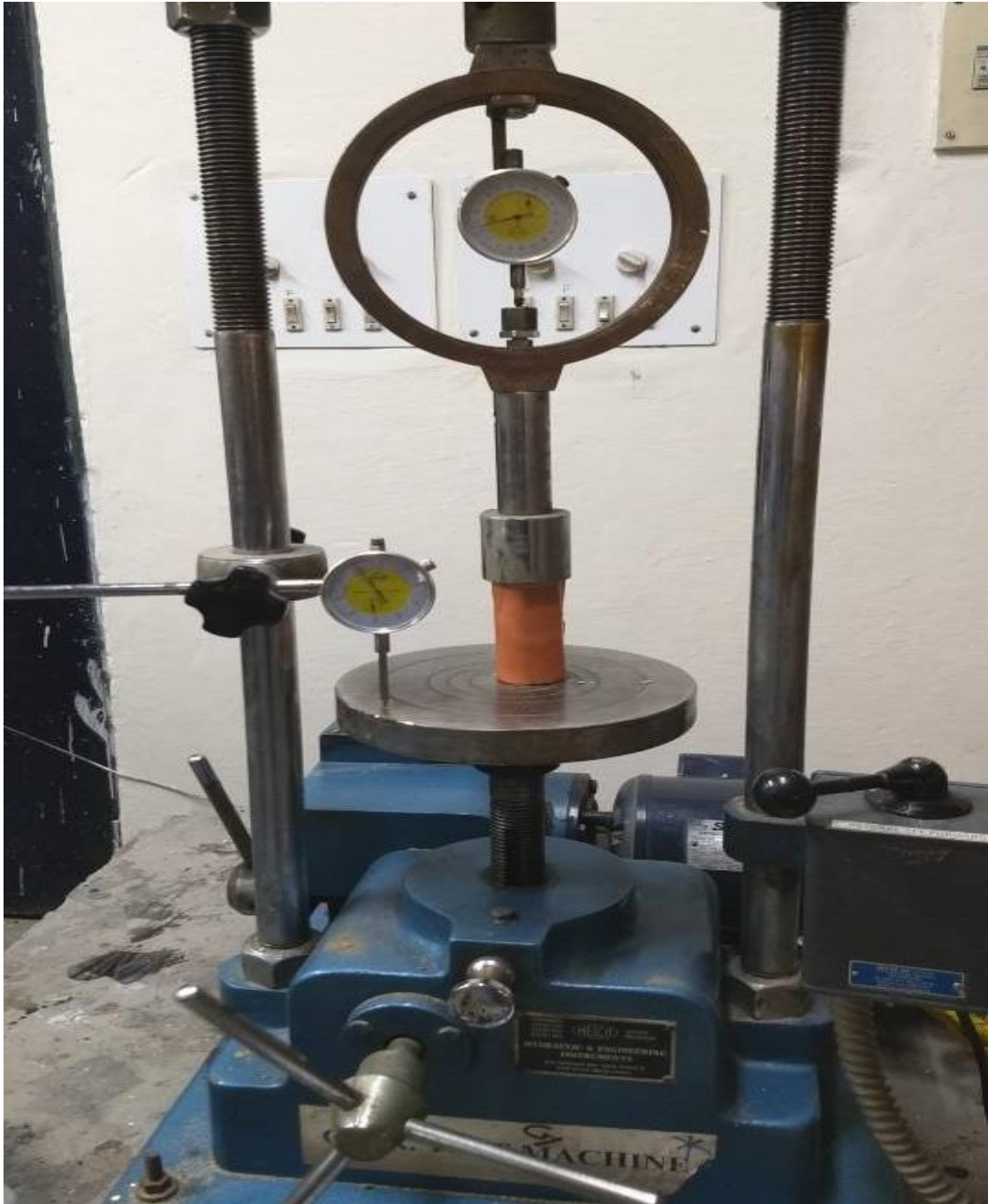
Figure 3.1.3: Uniaxial compression test for jointed rock specimen
