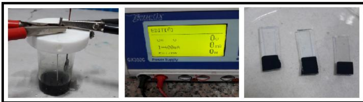
Figure 4.3- Electrophoretic deposition of PANI films using two electrode system on ITO
