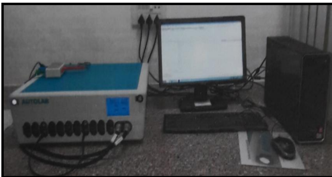
Figure 4.6- Autolab Potentiostat/Galvanostat, EcoChemie, Netherlands
