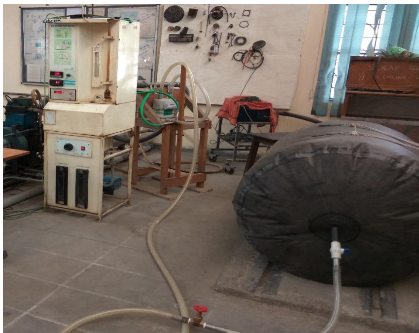
Fig.3.12 Biogas supply and metering system
