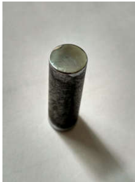
Fig 13: Chrome Coated Pin
