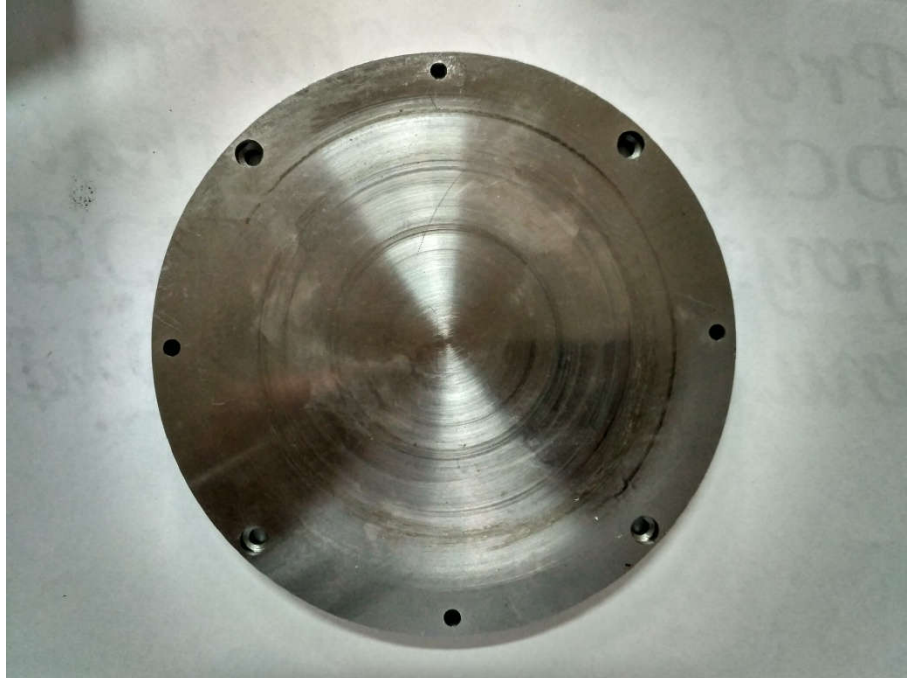
Fig 12: Mild Steel Disc
