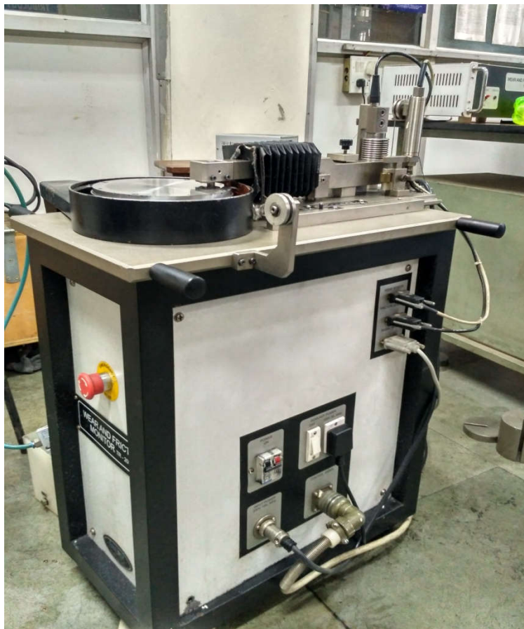
Fig 19: Pin on Disc Tribotester
