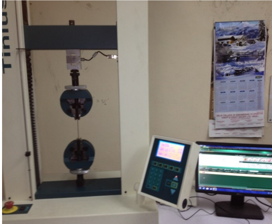
Fig. 4.2 50kN-UTM-table top in Metal Forming Lab. at DTU
