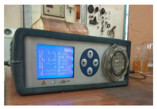
Figure 7: A view of AVL DIGAS 444, a gas analyser
