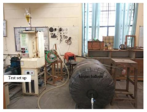
Figure 5: biogas supply system
