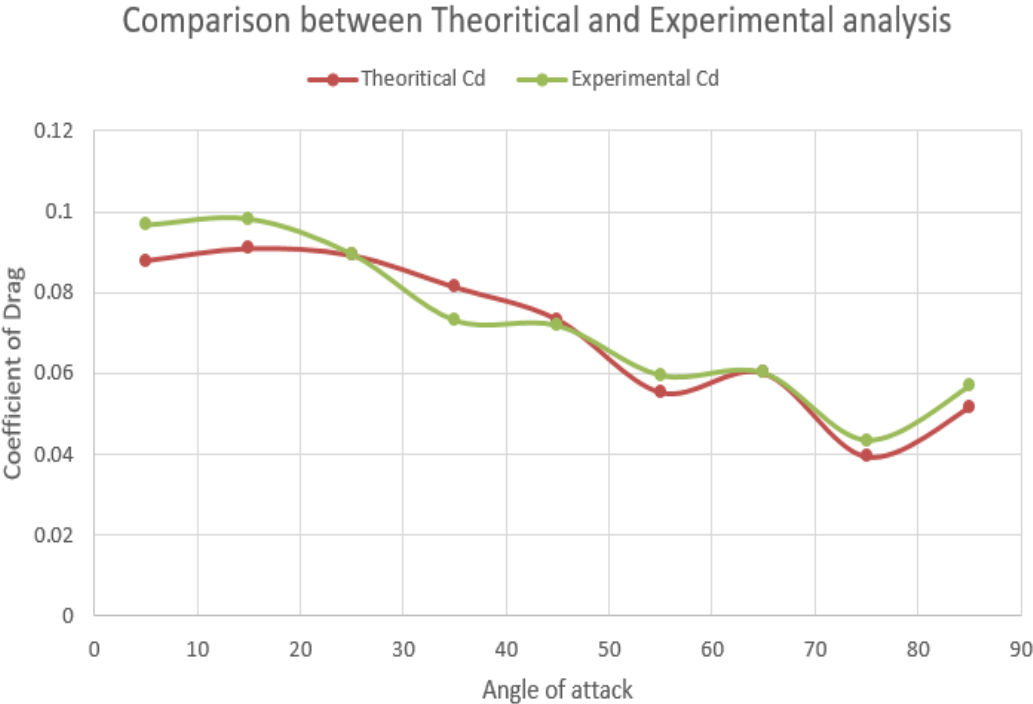
Figure 5.1 Validation for Angle of attack vs Coefficient of Drag at Re= 600000
