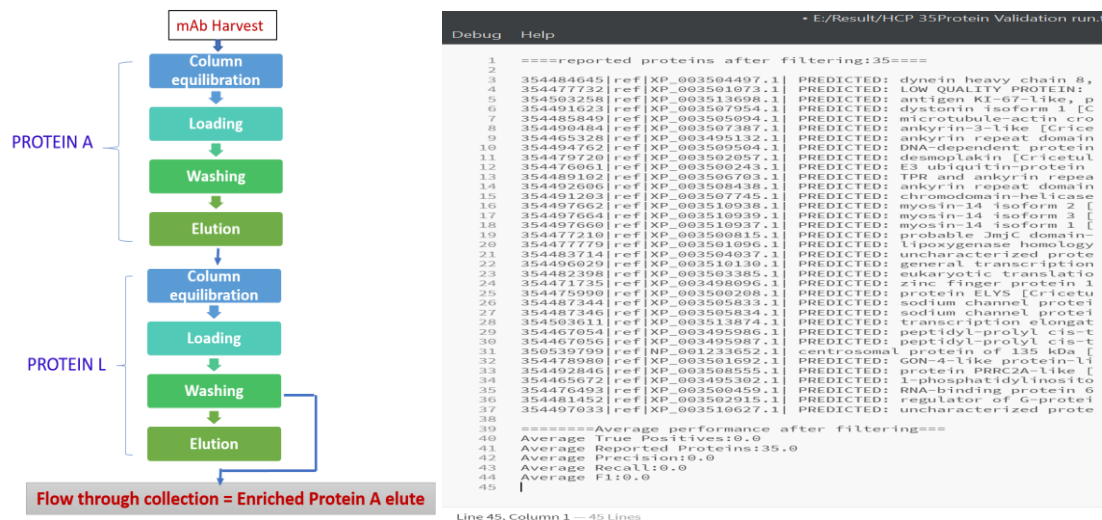
Figure 2: Steps involved in mAb purification and different HCP's being reported after washing and filtration
