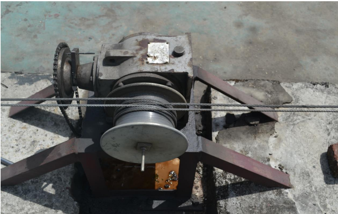
Fig.4.6: Drive mechanism using DC wiper motor of 12V and Chain sprocket assembly
