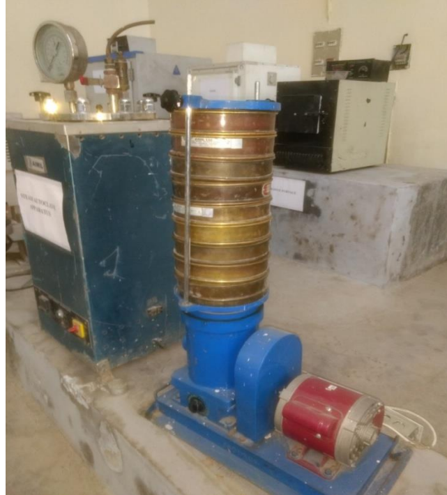
Fig. 3.9: Sieve shaking of coarse sand
