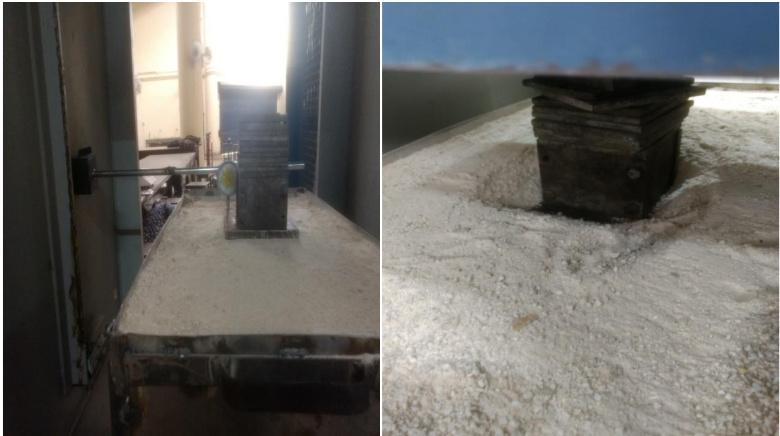
Fig. 3.13 (a) Arrangement of setup for performing plate load test
