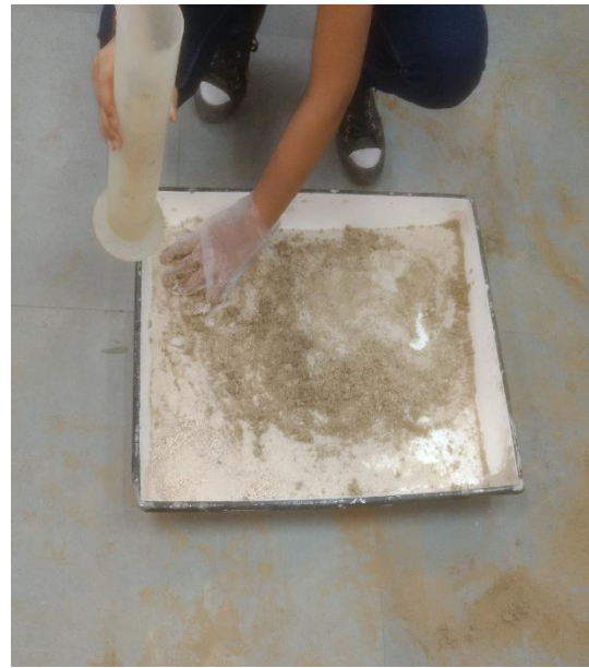
Fig. 3.10 (a) Mould filled with the coarse sand
