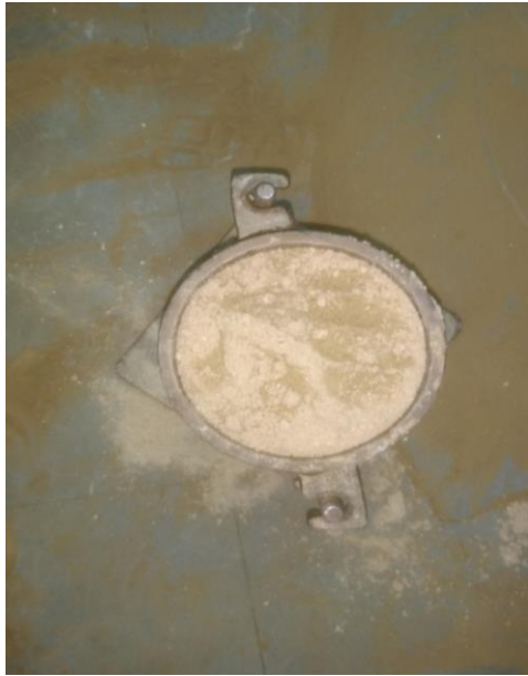
Fig. 3.10 (a) Mould filled with the coarse sand
