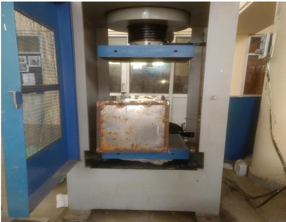
Fig.3.6: Placed MS steel box in ACTM machine
