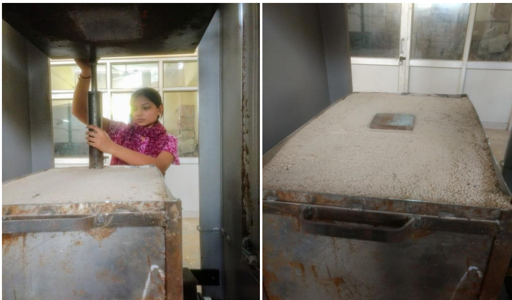
Fig.3.12: (a) Providing number of blows to sand for increasing its density (b) Placement of square plate over the top of soil
