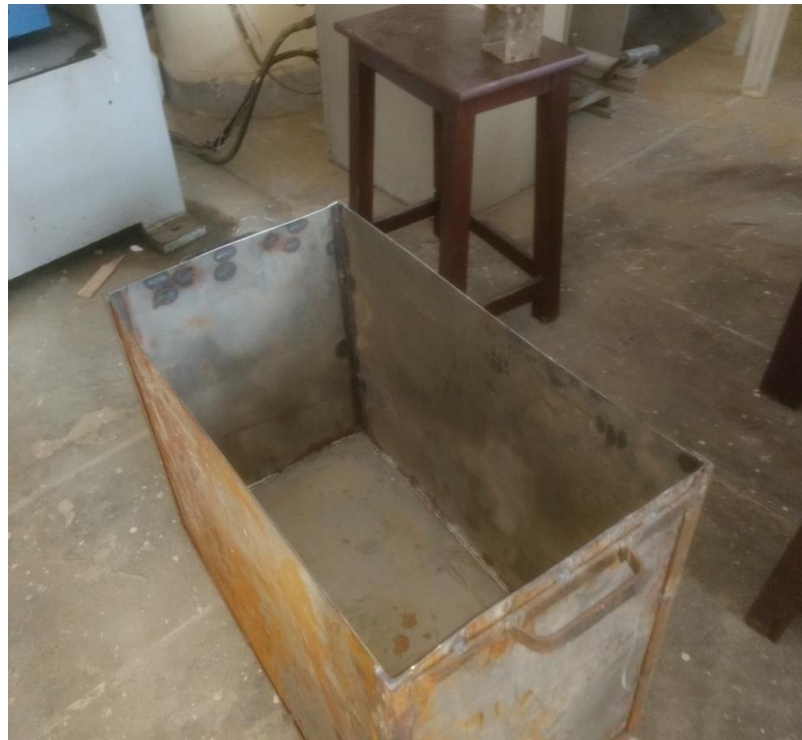
Fig.3.3. (a) M.S steel box of size 40mm x 70mm x 50mm
