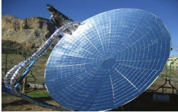
Figure23: - collector of solar paraboloid dish (source: - NREL)
