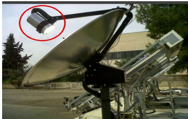
Figure24: - cavity receiver of solar paraboloid dish (source: - NREL)
