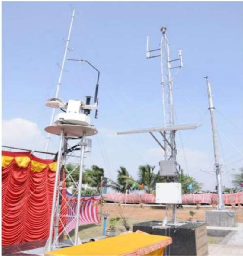
Figure11: - solar radiation resource assessment station (source: - NIWE)
