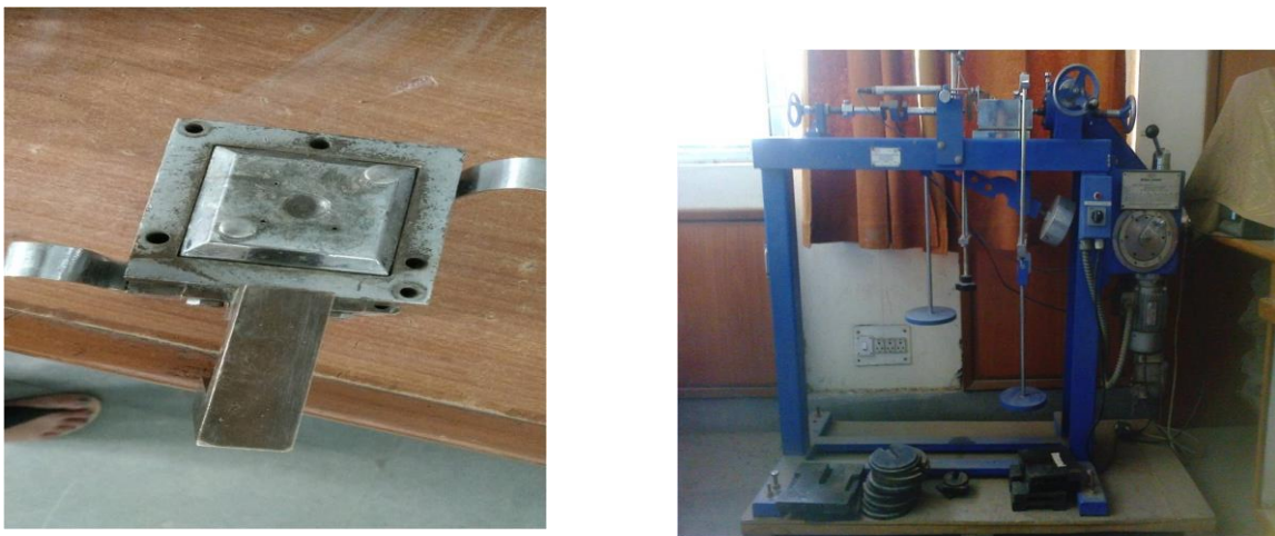
Figure3.8. Shear box and Direct shear apparatus
