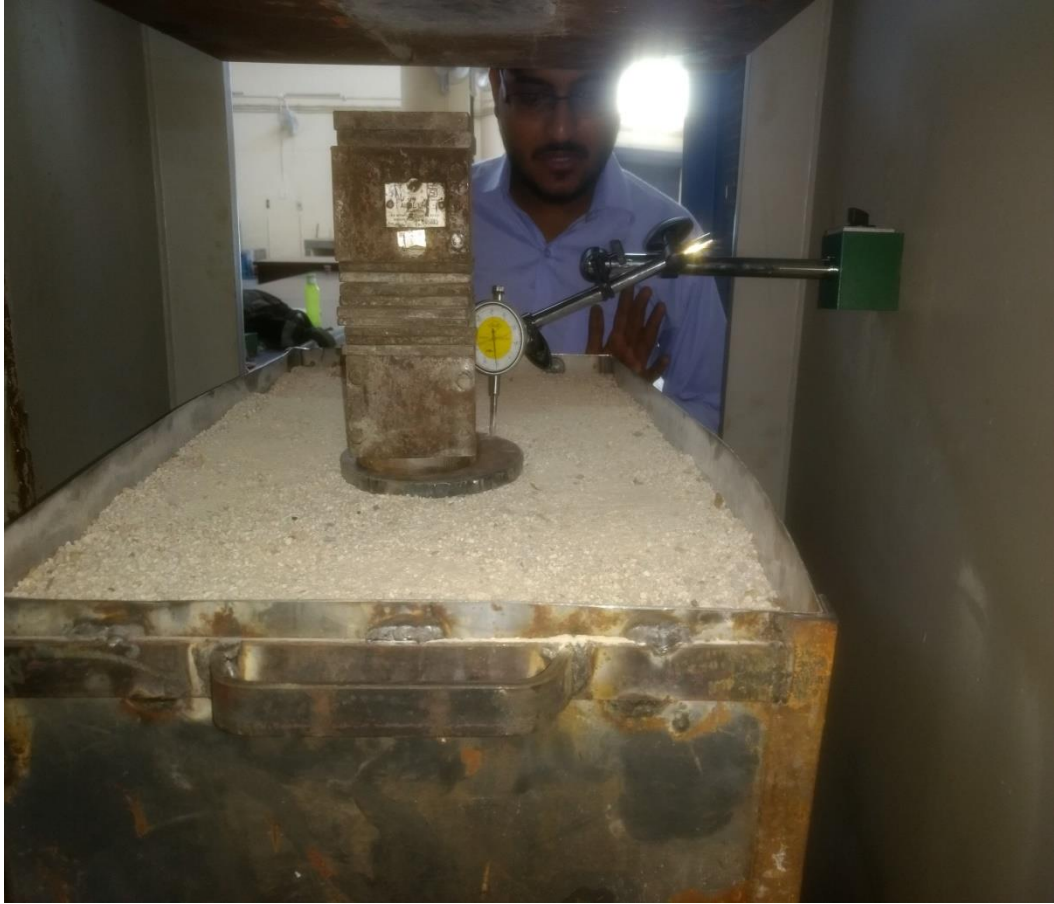
Figure3.10. Setup of dial gauge and plate
