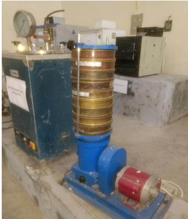
Figure3.6. Sieve analysis in sieve shaker
