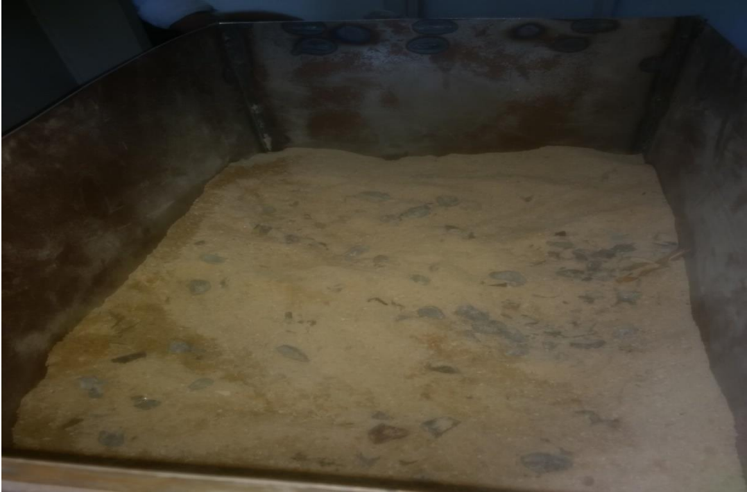
Figure3.12. Mixture of sand and fine gravel
