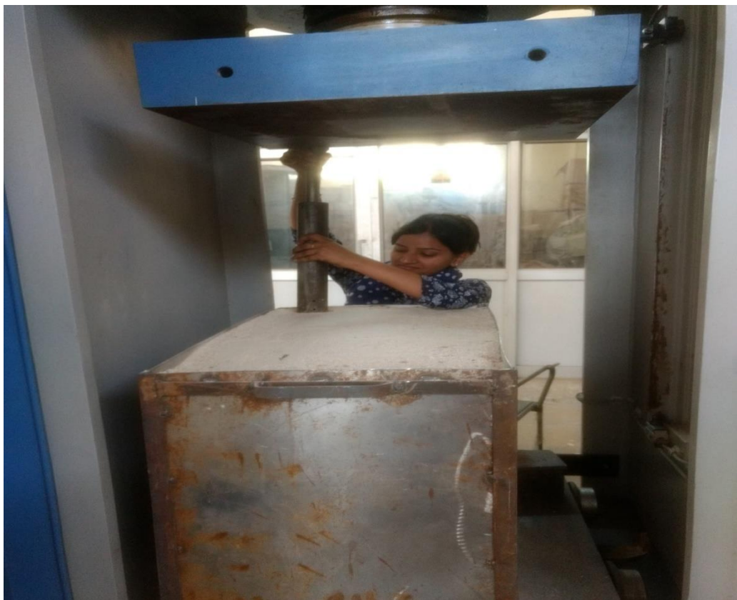
Figure3.9. Densification of sand using rammer
