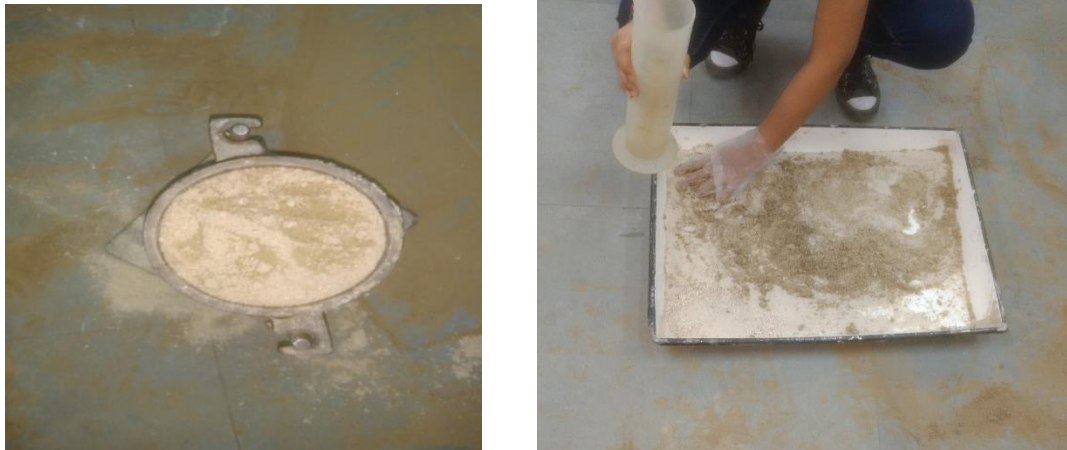
Figure 3.7 Standard proctor test
