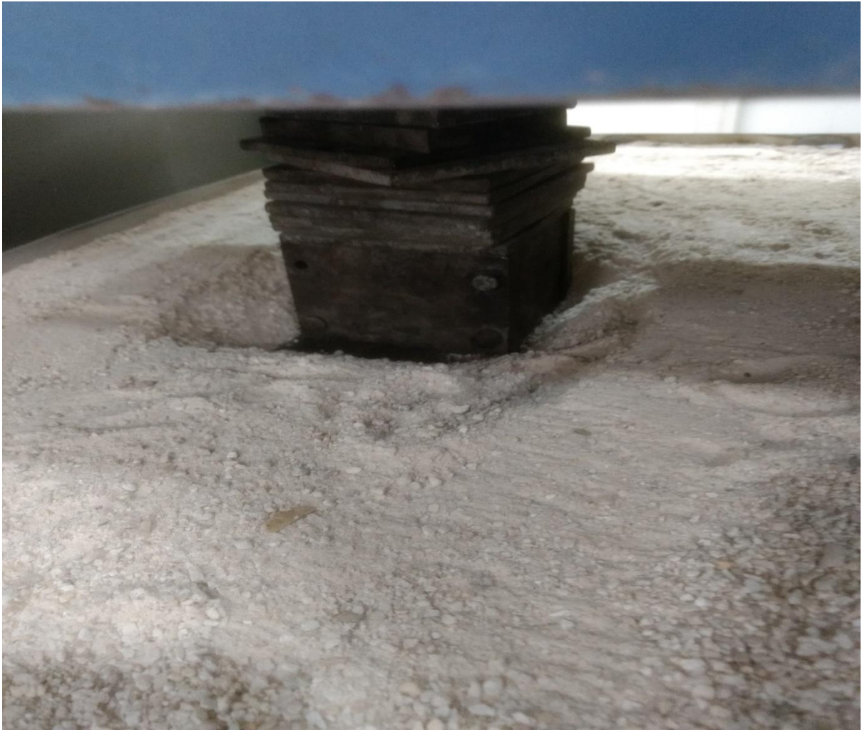
Figure3.11. Plate load test in compression testing machine
