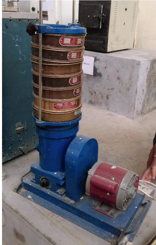
Photograph No. 2: Arrangement of sieve on the sieve shaker
