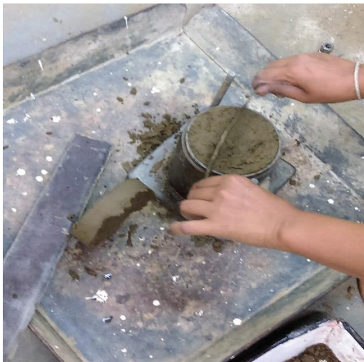
Photograph No. 4: Process of compaction test
