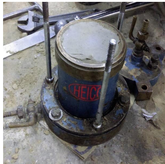
Photograph No. 10: Process for sample preparation for hydraulic conductivity test.
