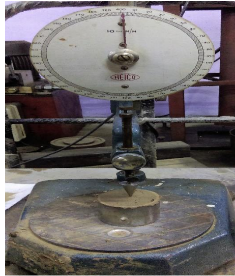
Photograph No. 3: Process of liquid limit test using cone penetrometer
