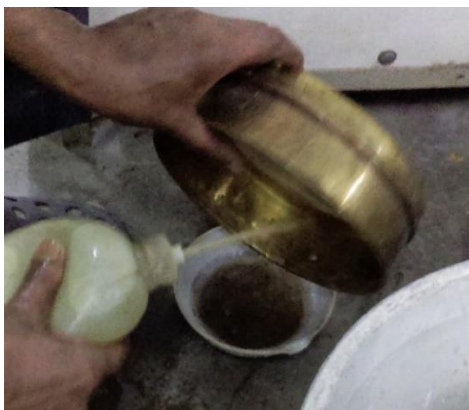
Photograph No. 1: Process of wet sieve analysis
