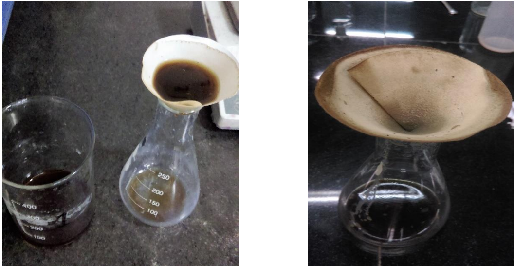
Photograph No. 6: Arrangement to find suspended solids.
