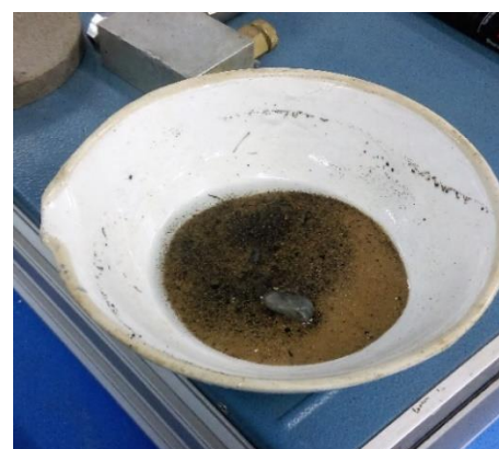
Photograph No. 1: Process of wet sieve analysis
