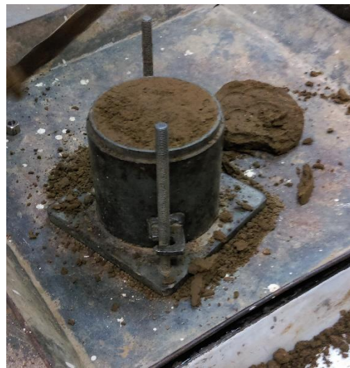
Photograph No. 4: Process of compaction test
