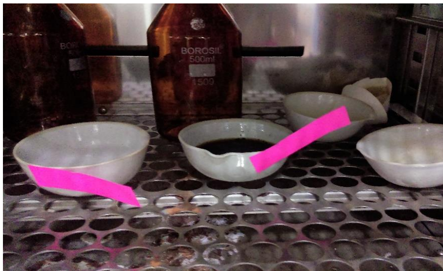
Photograph No. 5: dish with leachate kept in oven for determination of dissolved solids
