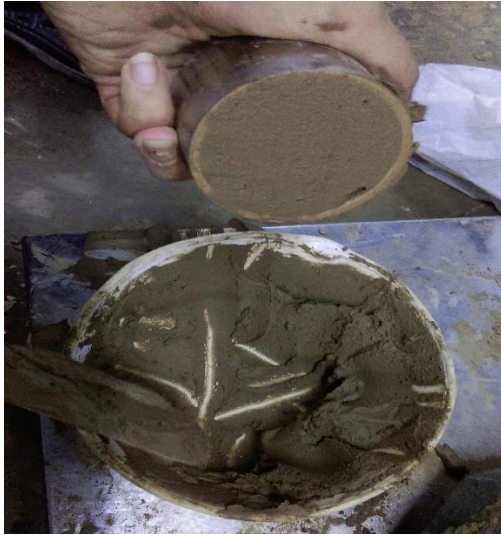
Photograph No. 3: Process of liquid limit test using cone penetrometer
