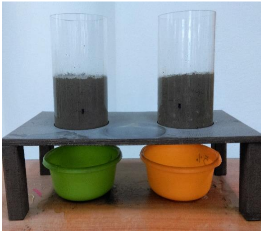
Photograph No. 11: Sample preparation and setup of the column study
