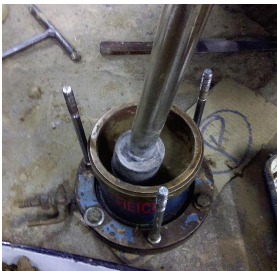
Photograph No. 10: Process for sample preparation for hydraulic conductivity test.
