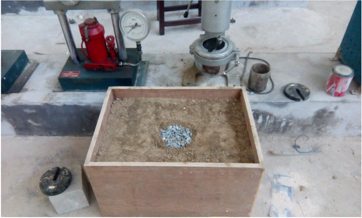
Figure 4.1. Stone Column Installed in Tank
