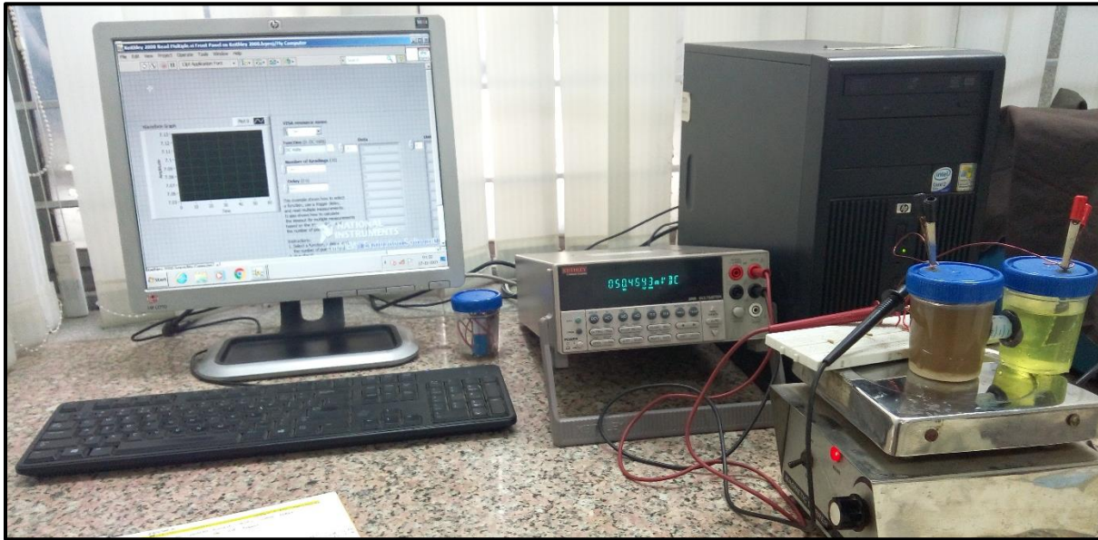
Figure 4.12 Keithley 2000 Digital Multimeter for current and potential measurement
