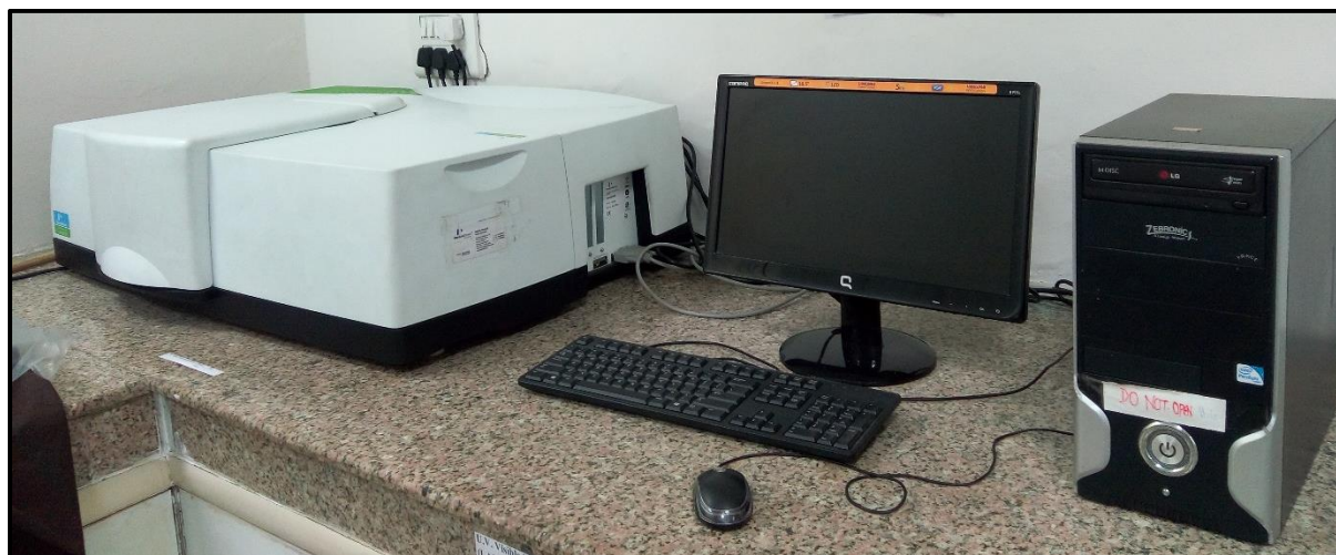
Figure 4.7(b) UV/Vis/NIR Spectrophotometer (Perkin Elmer Lambda 950)
