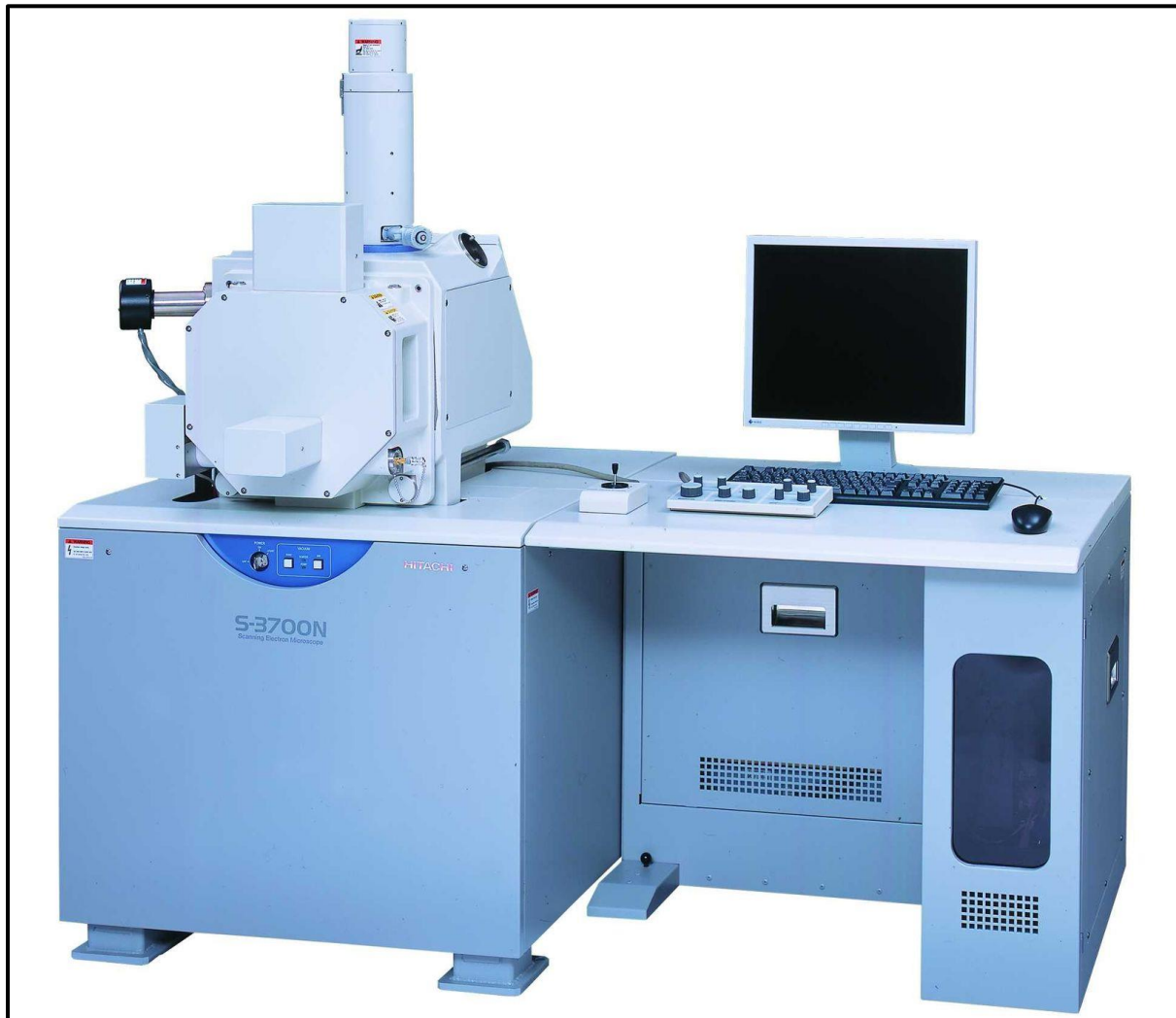
Figure 4.6 Scanning Electron Microscope (Hitachi S-3700N)
