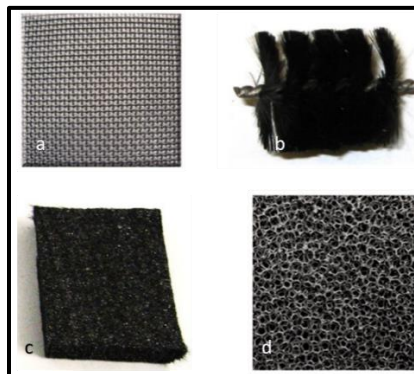
Figure 3.4 (a) Stainless Steel Mesh (b) Carbon Brush (c) Graphite felt (d) Reticulated vitrified carbon
