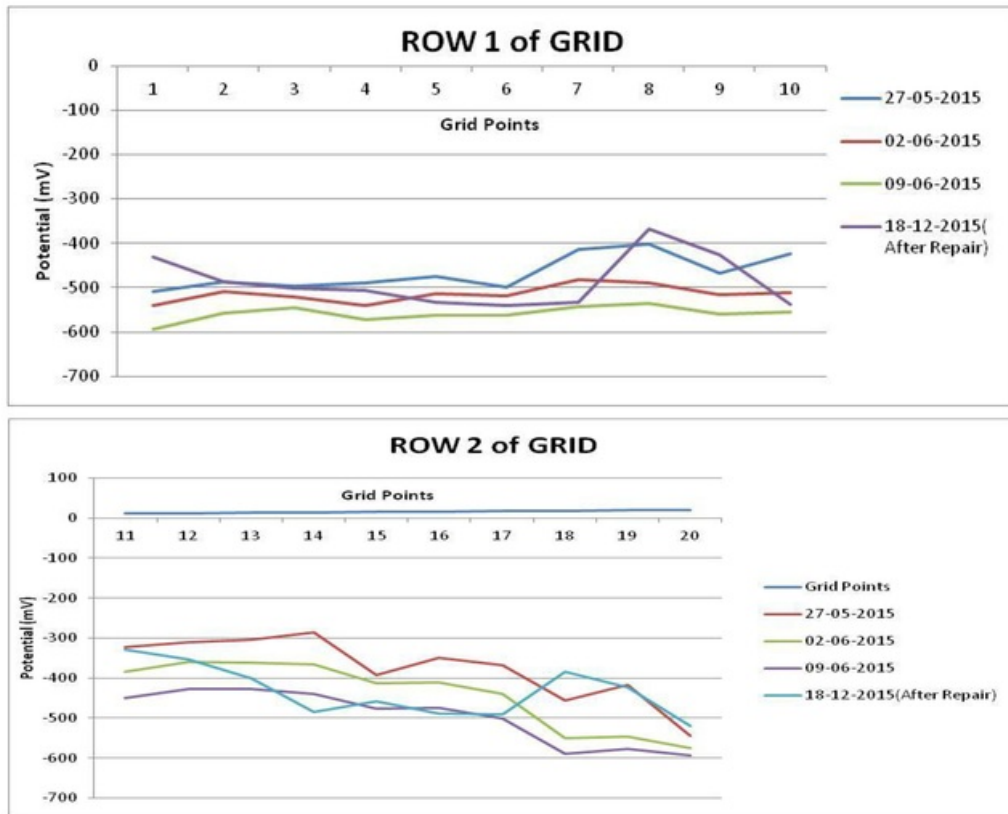
Figure 20: Graphical representation showing variation of potential before and after repairing of beam member.
