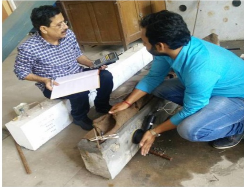
Figure 18: Measuring of OCP of reinforcement bar in beam
