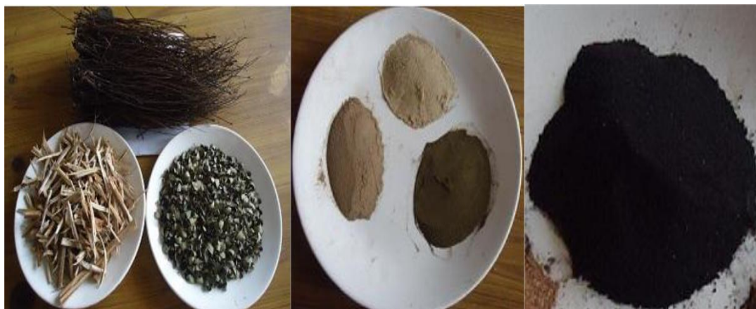
Figure.3.1: Specimen of biomass element, element powder & coal powder
