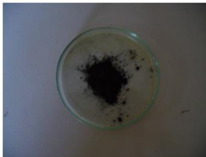
Fig 3.6 Solid carbon residue obtained after cracking
