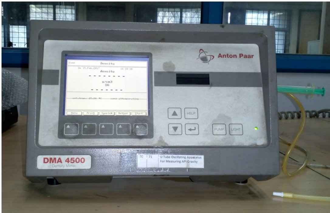
Fig 3.7: U-Tube Oscillating True Density meter
