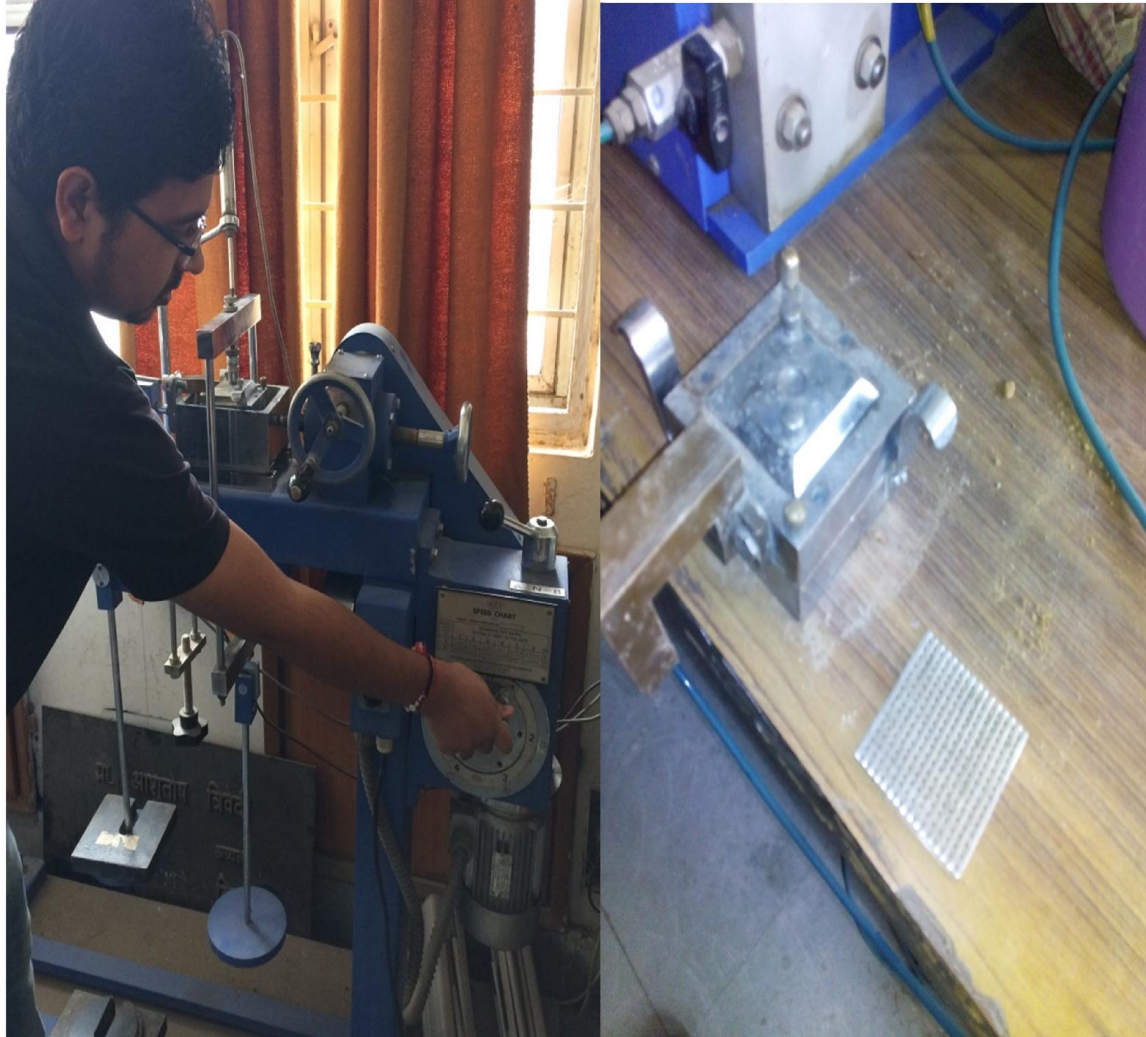
DIRECT SHEAR TEST MACHINE AND DIFFERENT PARTS OF SHEAR BOX
