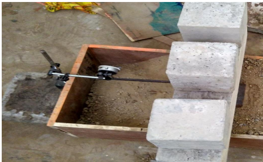
Fig 3.15 Loading on unreinforced soil slope.
