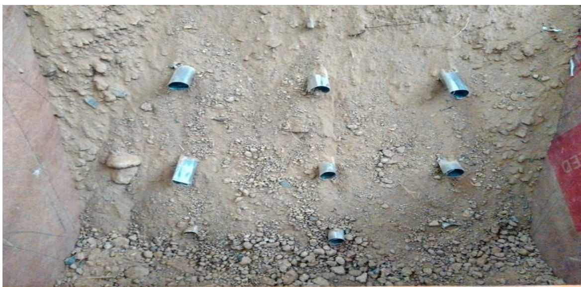
Fig 4.5 Aluminium hollow tubes inserted at 0^\circ to horizontal plane
