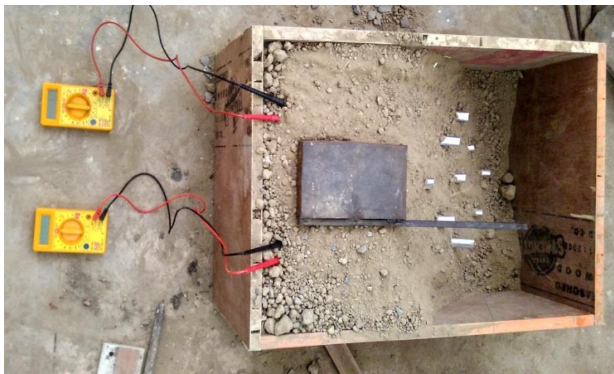
Fig 3.14 Soil nailed slope before loading
