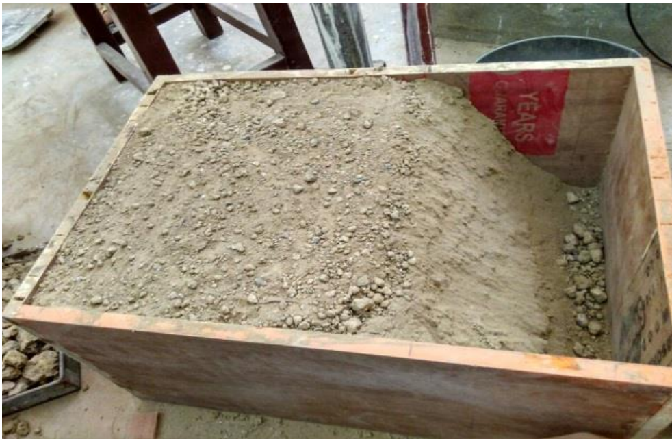
Fig 3.9 Unreinforced soil slope( 60^\circ )
