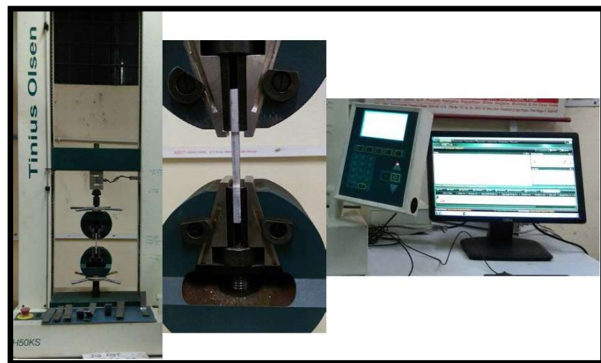
Fig. 3.13: Tensile Test Machine, Mounting, Control/ DAQ System (Left to Right)
