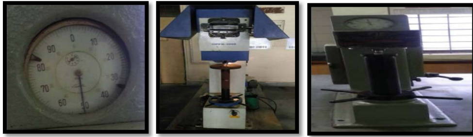
Fig. 3.12: Rockwell harness test machine, Rockwell no. indicator, Brinell hardness test machine (Left to right)
