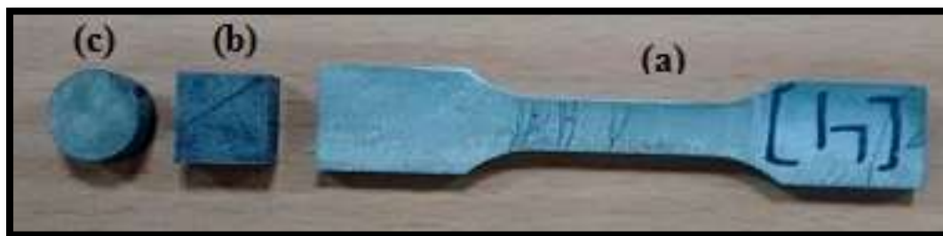
Fig. 4.4: Specimen from Plate shown above via EDM wire cut. (a) Tensile specimen, (b) Hardness and microstructure specimen, (c) Wear test specimen.
