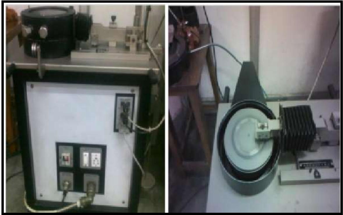
Fig. 3.14: Pin on disc Tribometer experimental setup
