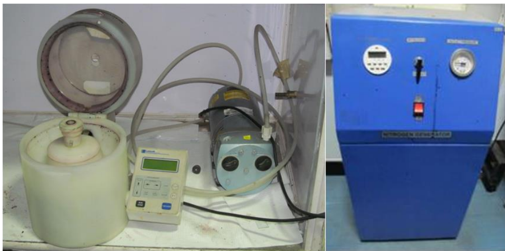
Figure 4.5 Picture of Spin Coating System in NPL, New Delhi
