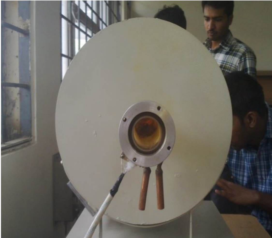
Plate 9 Micro Processor Controlled Furnace Inlet section
