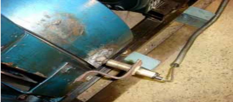
Plate 26 Digital Tachometer used for rpm measurement
