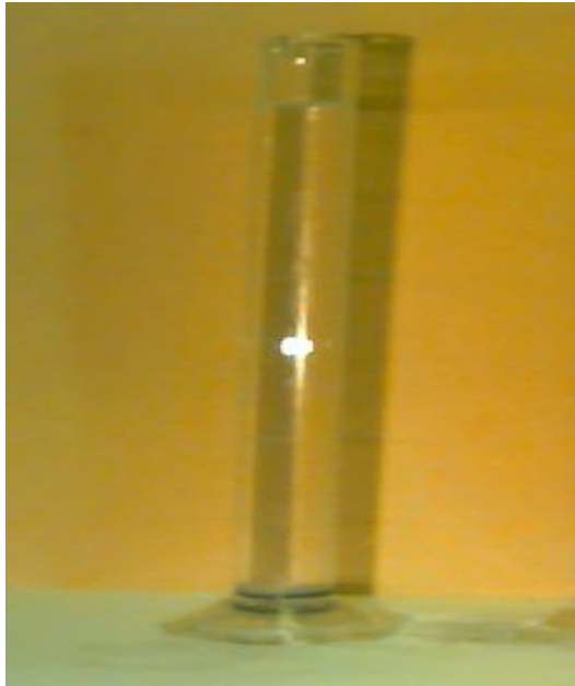
Plate 13 Showing the stable suspension of alumina nano particles in the diesel fuel
