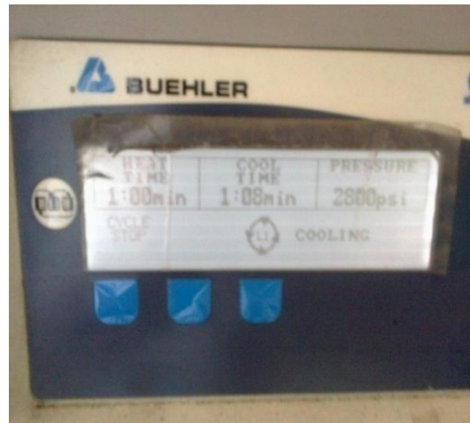
Figure 3.8 Heat time and cool time of Automatic Mounting press.
