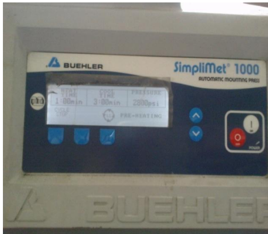
Figure 3.8 Heat time and cool time of Automatic Mounting press.
