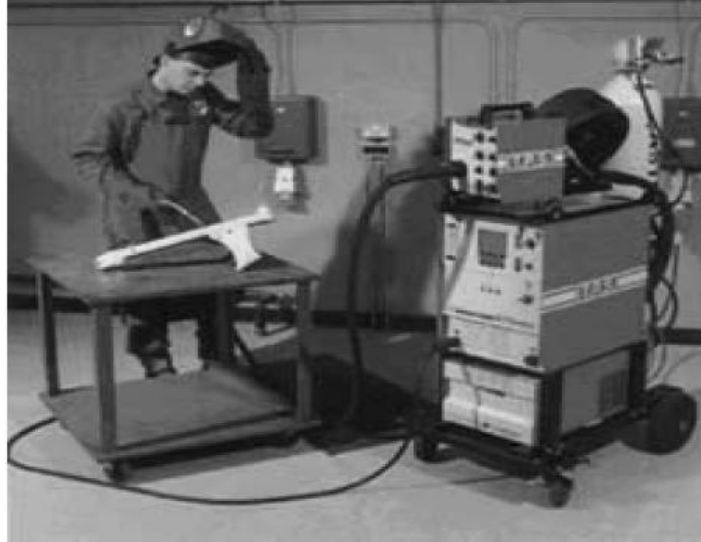
Figure: 3.2 General arrangement of the power source, wire feeder gas cylinder and work area
