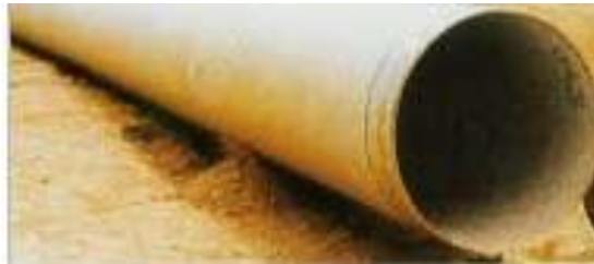
Fig A1.1: Photograph of GRP pipe.
