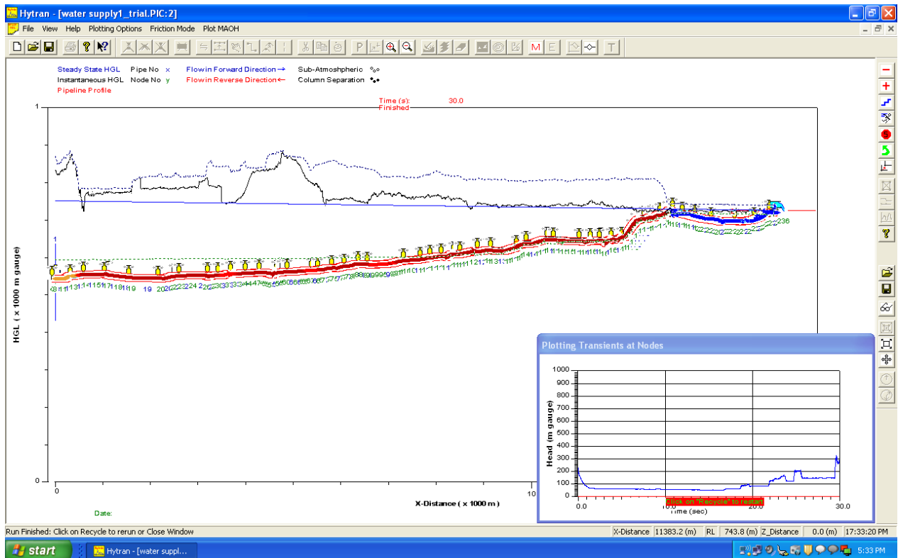
Fig 4.13: Transient analysis in Hytran software showing negative pressure zones in red ( Simmar WSS)
