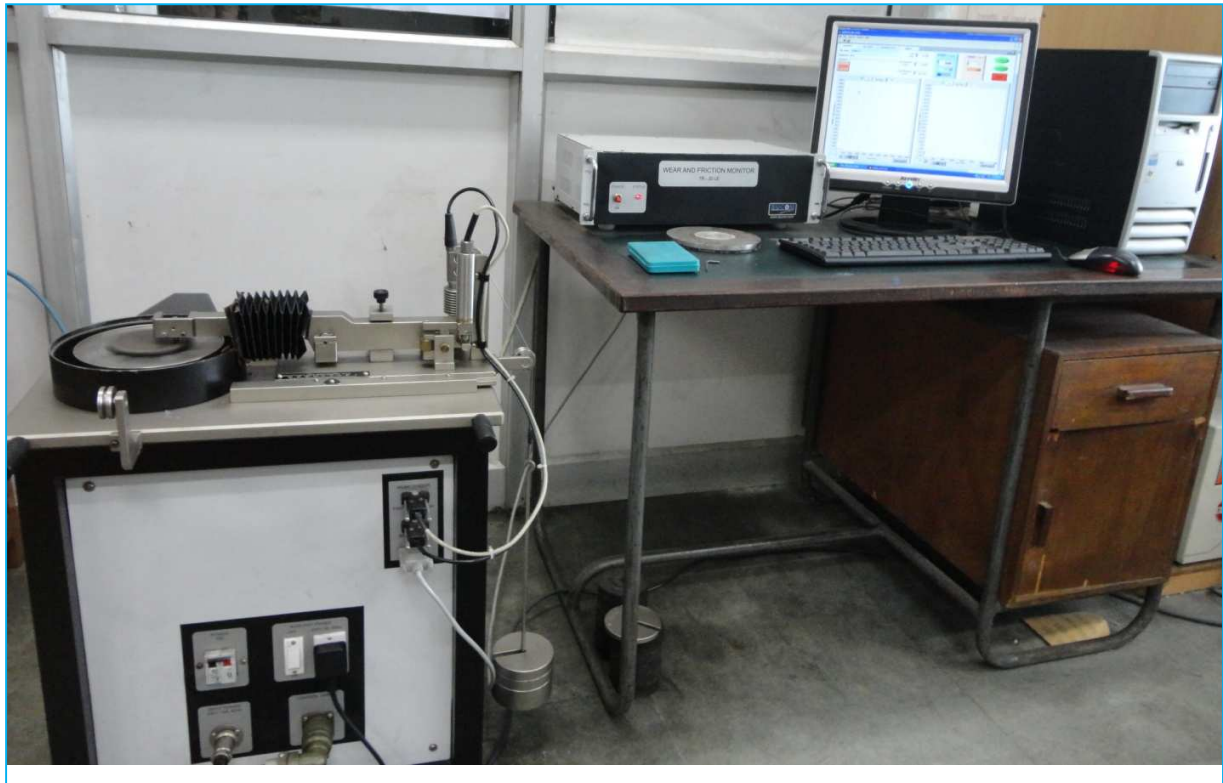
Figure 3.5- Wear and friction monitor machine for pin on disc test
