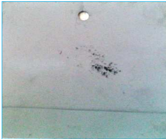
Figure 3.6 Ion Plated Disc before wear test
