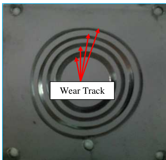
Figure 3.8 – Ion Plated Specimen after wear test
