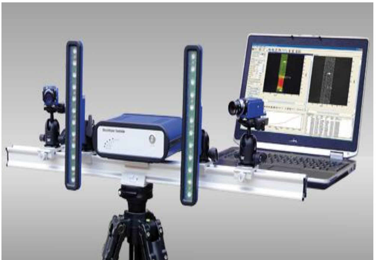
Figure 3.1 Setup containing various important component of DIC
