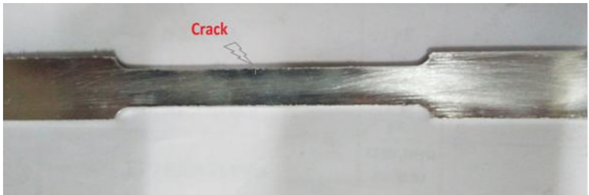
Figure3.5 : Specimen 2 (with crack without hole)
