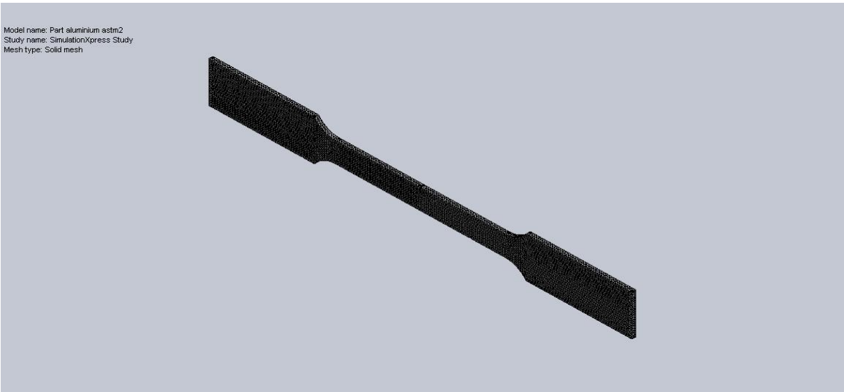
Figure3.17 : Showing model of specimen 2 after meshing
