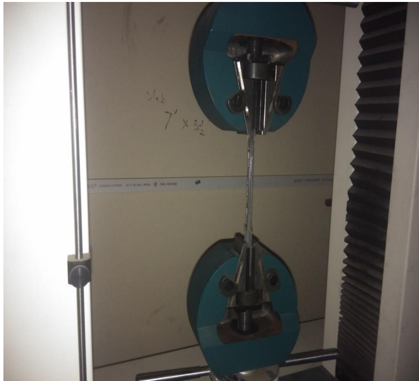
Figure3.8: UTM loaded with specimen
