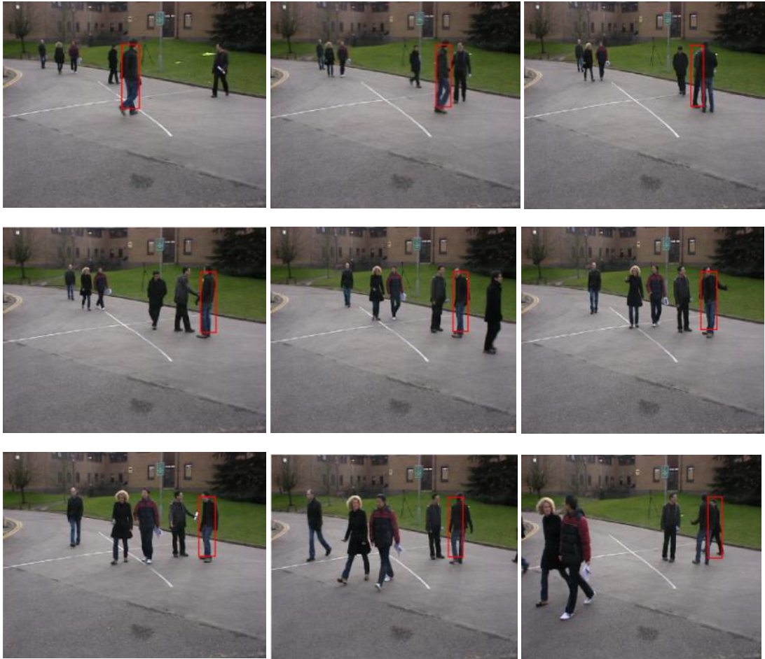
Figure 6.2: Frame number 10 to 100 in multiple of 10 from left to right respectively, showing the tracking of an object without the consideration of the background reference points.
