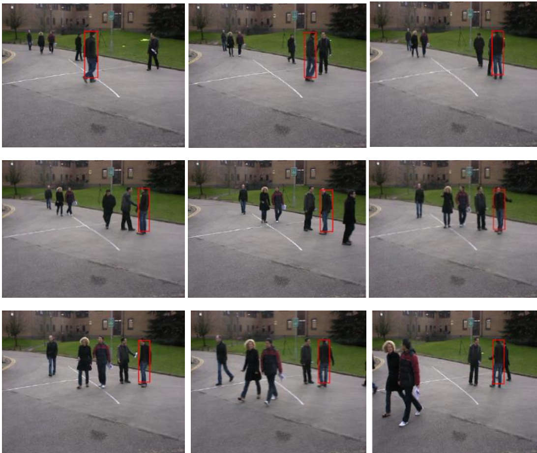
Figure 6.1: Frame number 20 to 100 in multiple of 10 from left to right respectively, showing the tracking of an object with the consideration of the background reference points.
