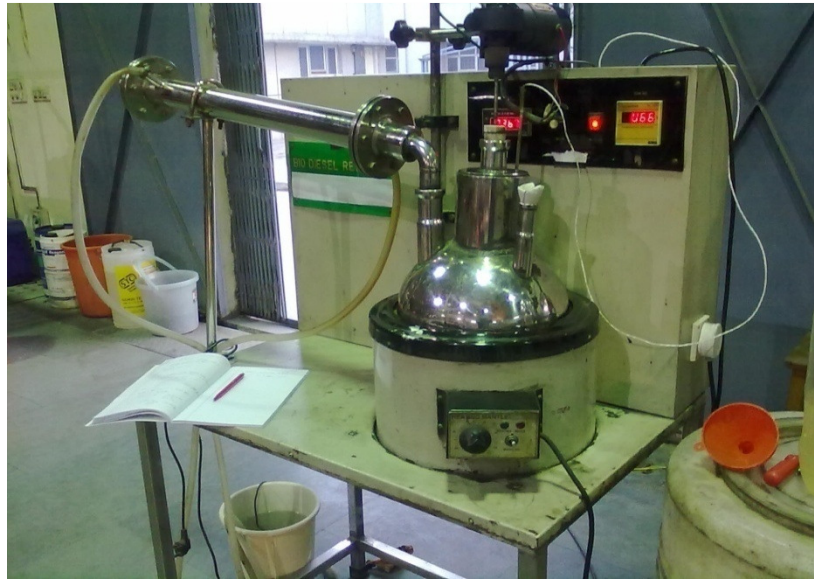
Plate 3.1:- Biodiesel reactor(10 litre capacity)
