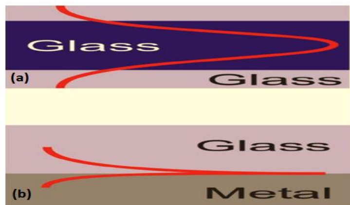
Figure 1.8 Confinement of light in (a) photonic and (b) plasmonic waveguide.
