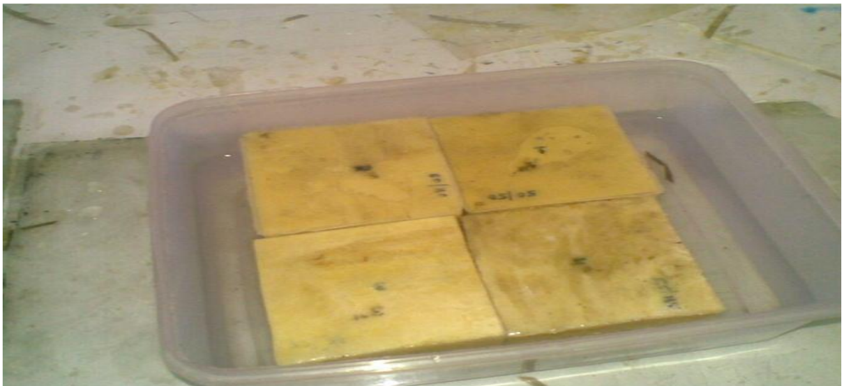
Figure 4.21: Water Absorption Test
