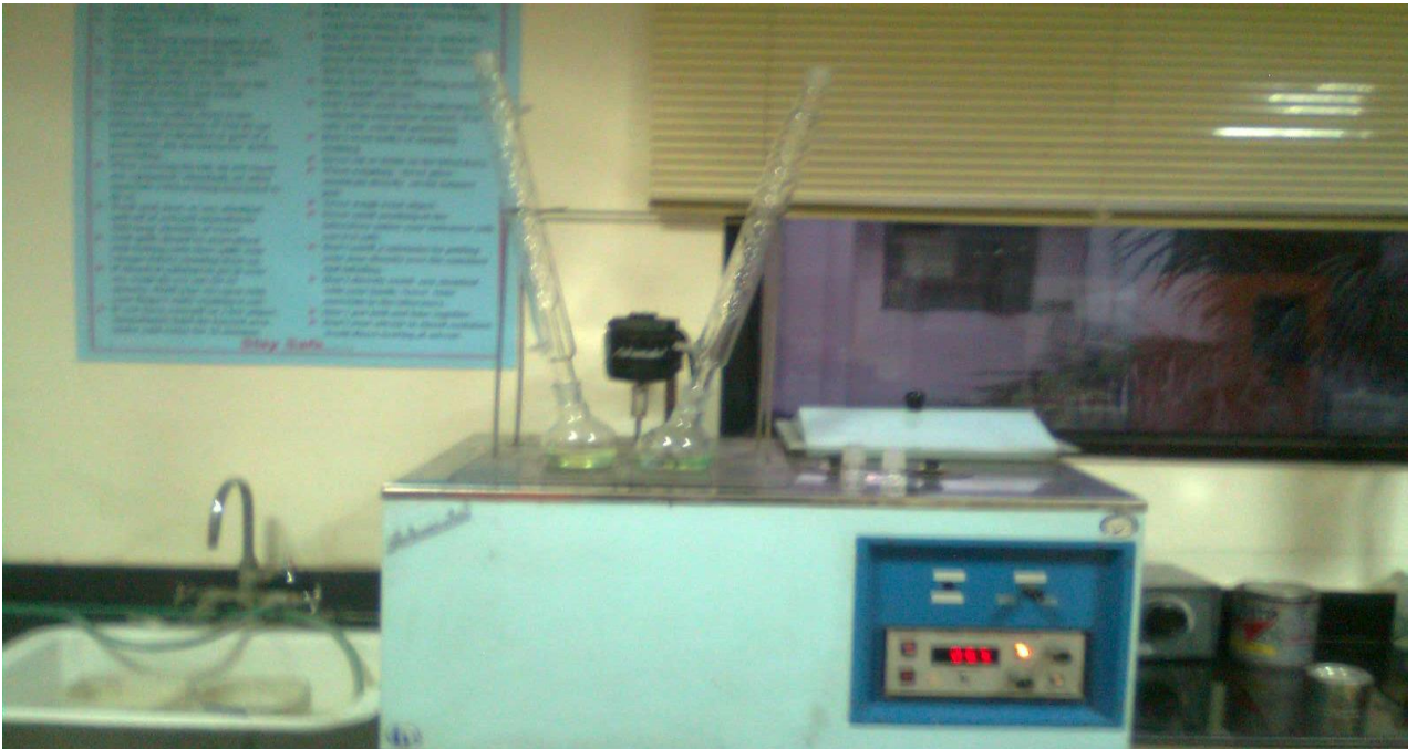
Figure A1.6: Water bath with Air Condenser
