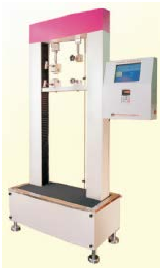
Figure 2.5: Universal Testing Machine (International Equipments)
