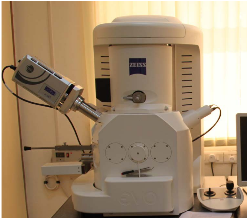
Figure 2.4: Scanning Electron Microscope (Zeiss EVO MA15)
