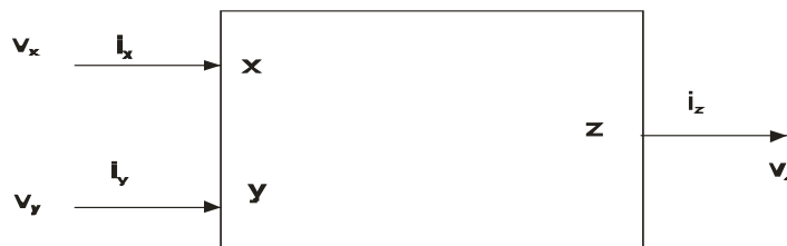
Fig5: Current Conveyor General Block Diagram
