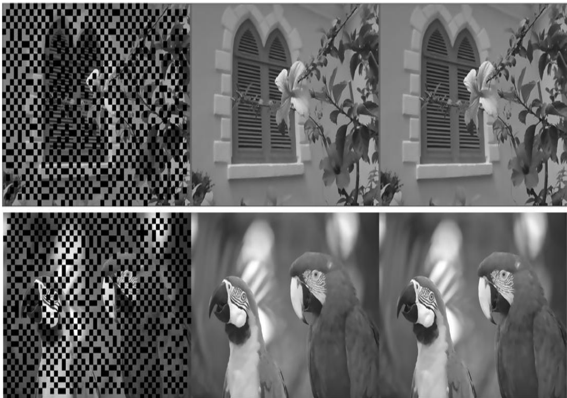
Figure 4.5 [16] image compression. First part shows the compressed image with black removed blocks rest of the blocks are encoded using image encoding techniques , second image shows the decoding with inpainting and third shows the image with normal encoding technique
