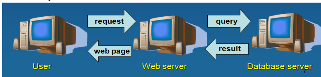
Fig.4 Schematics of Biological databases: Biological databases often have web interfaces, which allow users to send queries to the databases
