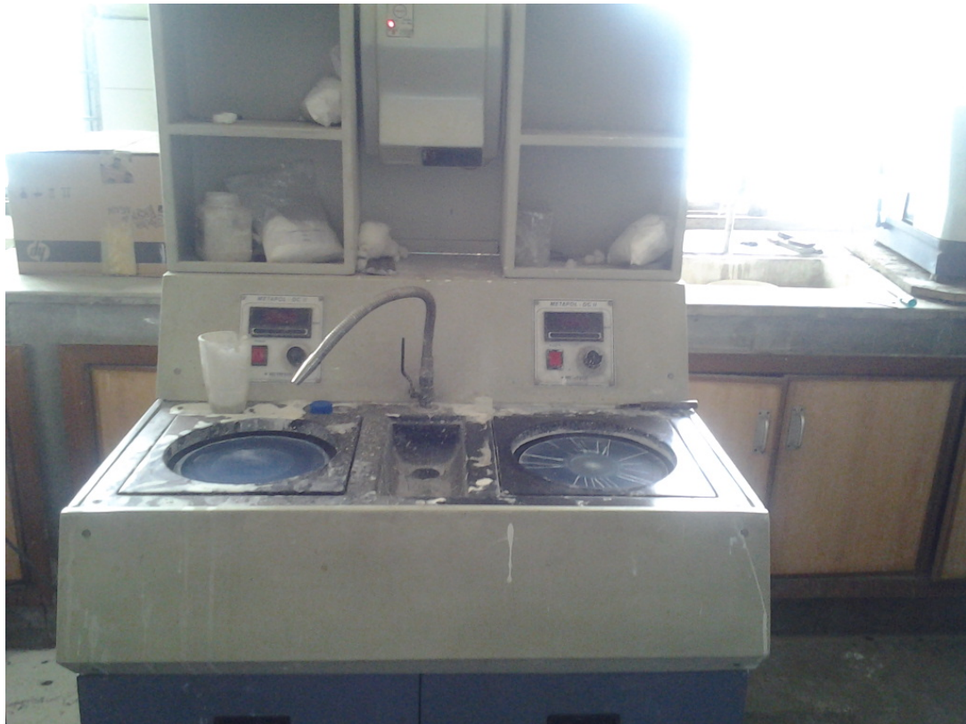
Figure 4.7 setup of machine for dry and wet polishing
