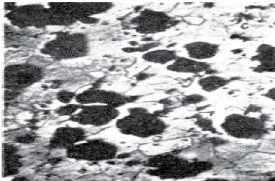
Figure 2.3 Microstructure of blackheart malleable cast iron [1]
