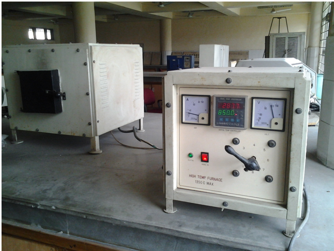
Figure 4.6 Electric furnace for post weld heat treatment
