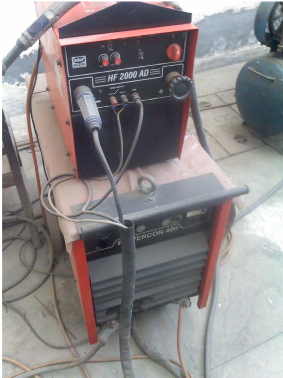
Figure 4.5 set up of shielded metal arc welding machine
