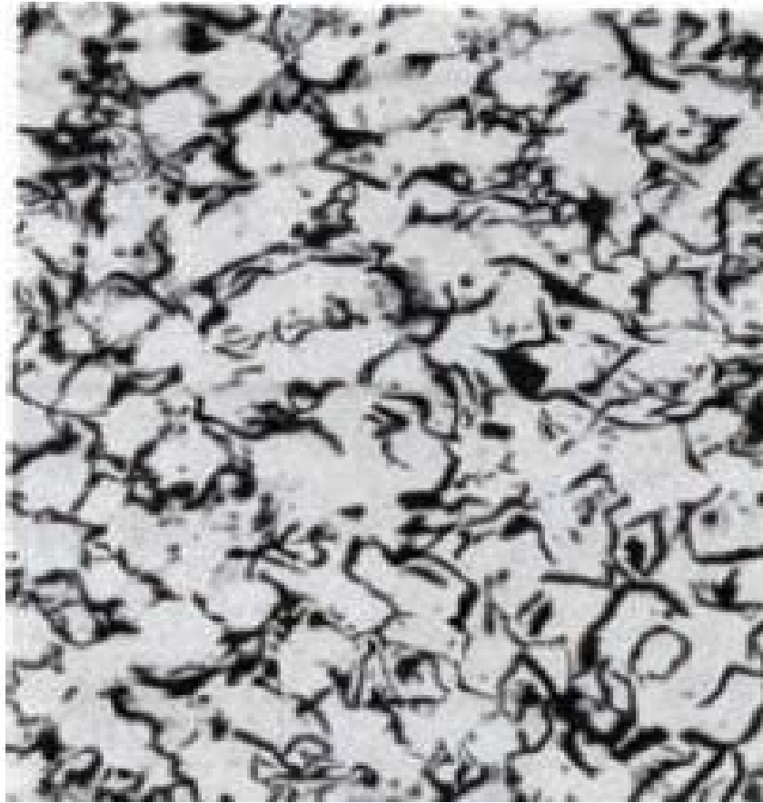
Figure 2.1 Microstructure of gray cast iron[1]
