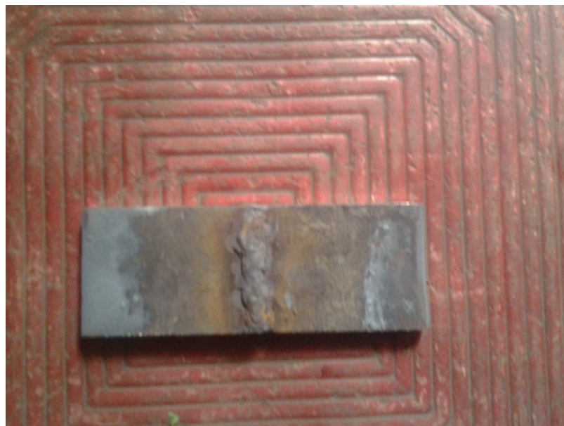
Figure 4.4 welded plate with PWHT
