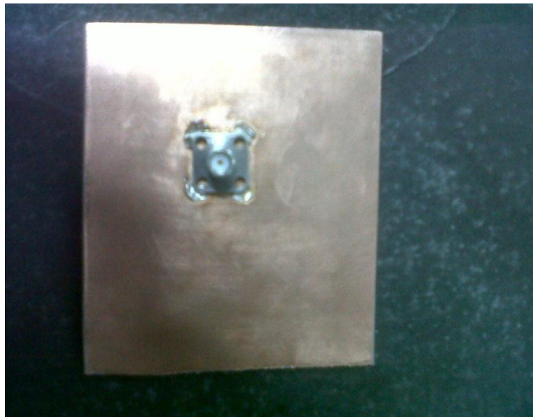
Fig.6.3 Fabricated antenna with Coaxial Connector
